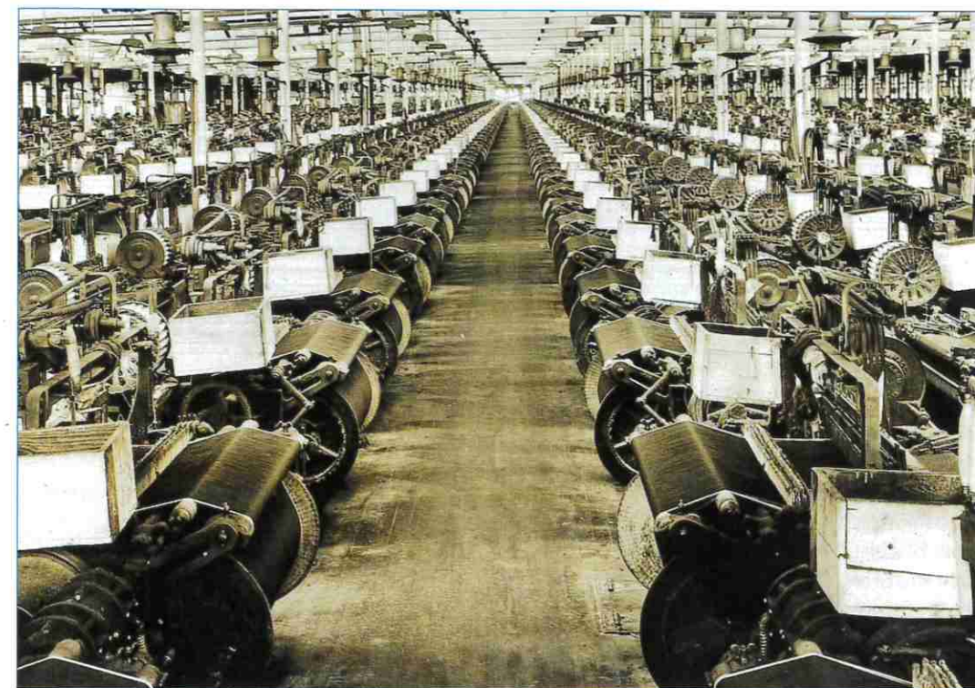
1940s photo of selvedge denim shuttle looms, taken from only halfway across the vast room.
