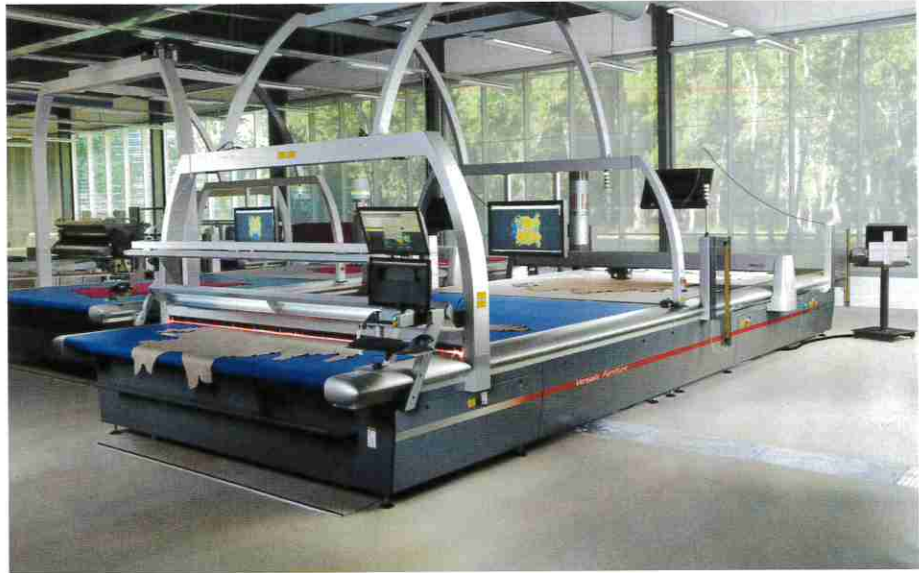
By using Lectra's Versalis automated leather cutting solution, Duvivier Canapés has been able to make significant improvements in productivity and cutting quality. CREDIT: LECTRA
