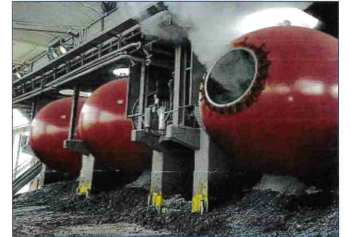
The thermal hydrolysis plant at Ilsa in Arzignano. This local biotech firm collects tannery waste and uses it to create added-value products such as fertilisers, keeping the Arzignano leather industry at the forefront of innovation.
