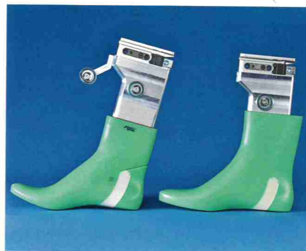
HPML lasts are compatible with automated production systems and Industry 4.0.
