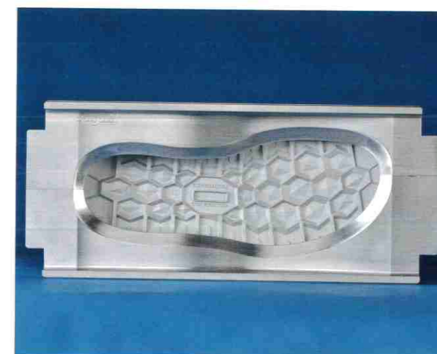
Five-axis machining is used to produce complex and highly details moulds.
