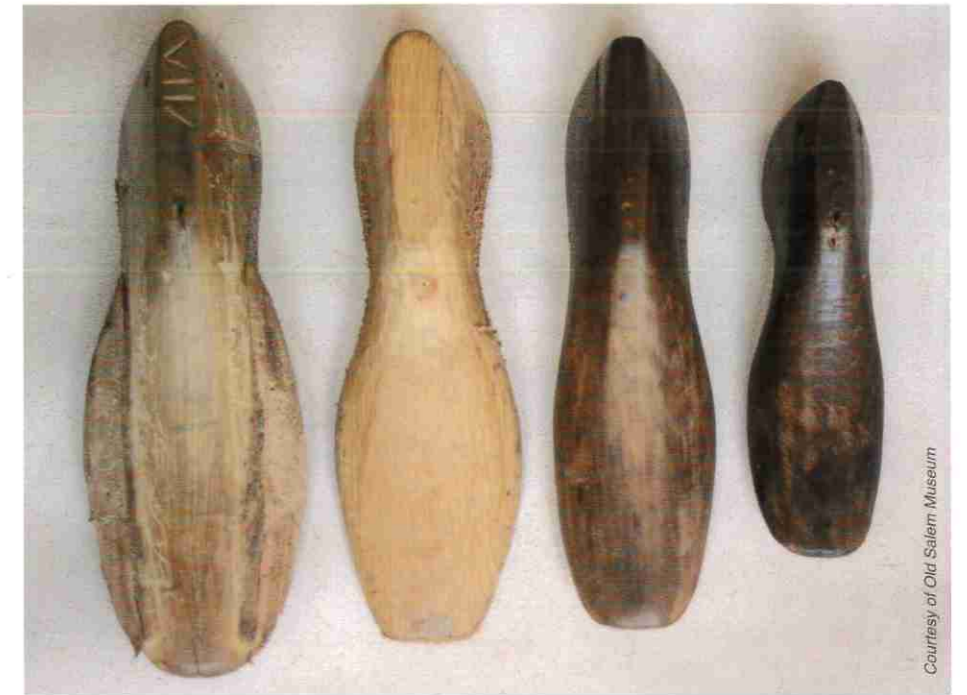
Figure 1: 'straight' lasts – with no difference between the left and the right foot – were used until the 1800s
