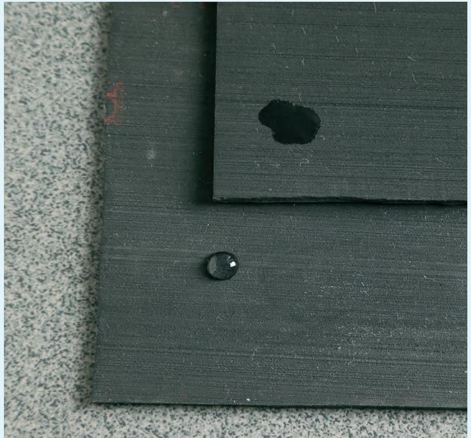
*Figure 2: The rubber surface (bottom) is untreated, so the water remains as a droplet without wetting the surface. The other sample (upper right) has been primed using solvent-free technology and the effect on the water is very apparent – the water now freely wets the rubber surface, essential when using water-based adhesives*
