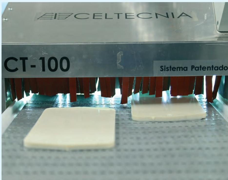
Figure 3: Moulded rubber slabs entering the Centecnia machine to prime the surface prior to the testing of bonds
