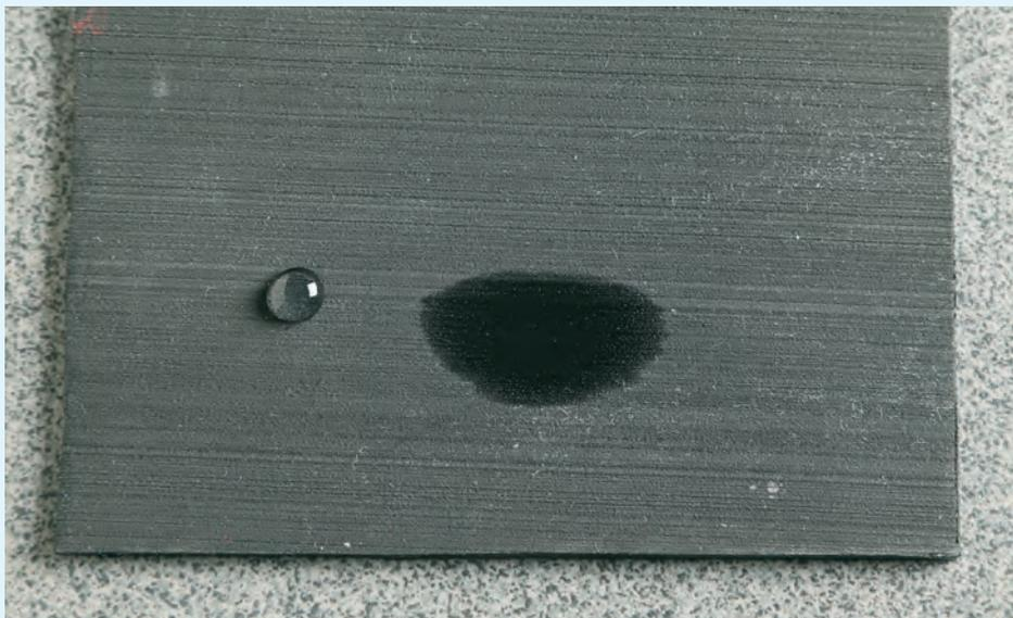
*Figure 1: As rubber has a low surface energy, the water droplet (left) is not wetting the surface due to its relatively high surface tension. By contrast, a solvent has a relatively low surface tension, and in this case easily wets the surface of the rubber (right)*
