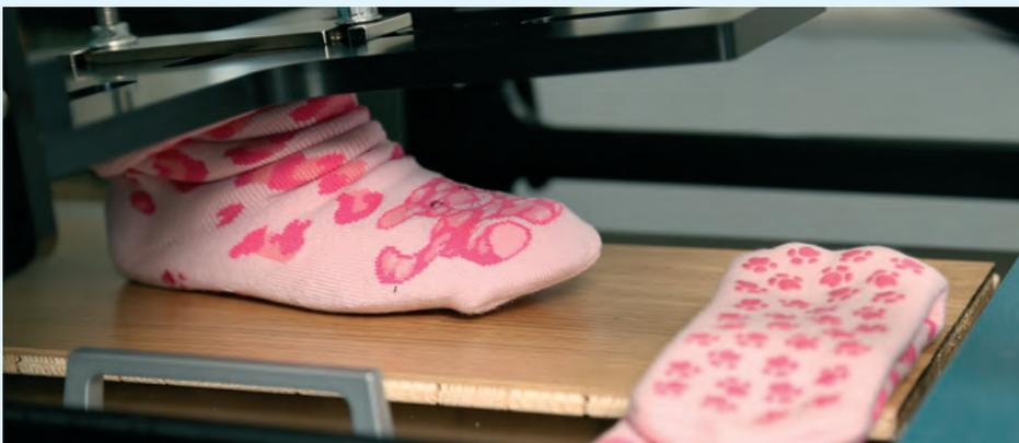
Using the SATRA TM144 test method to assess the slip resistance of a slipper sock
