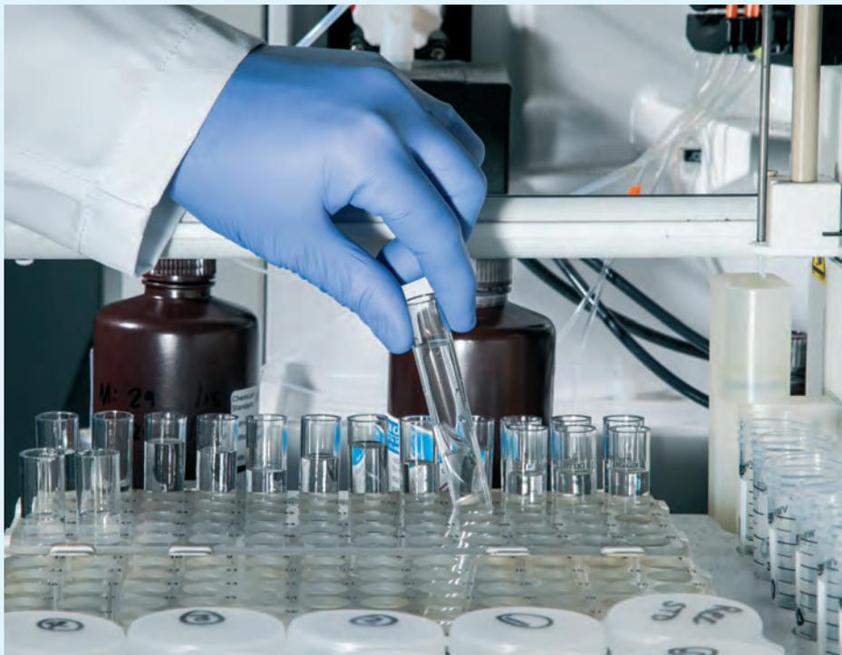
Extractable metals being measured by inductively coupled plasma (ICP) spectrometry in line with EN 71-3
