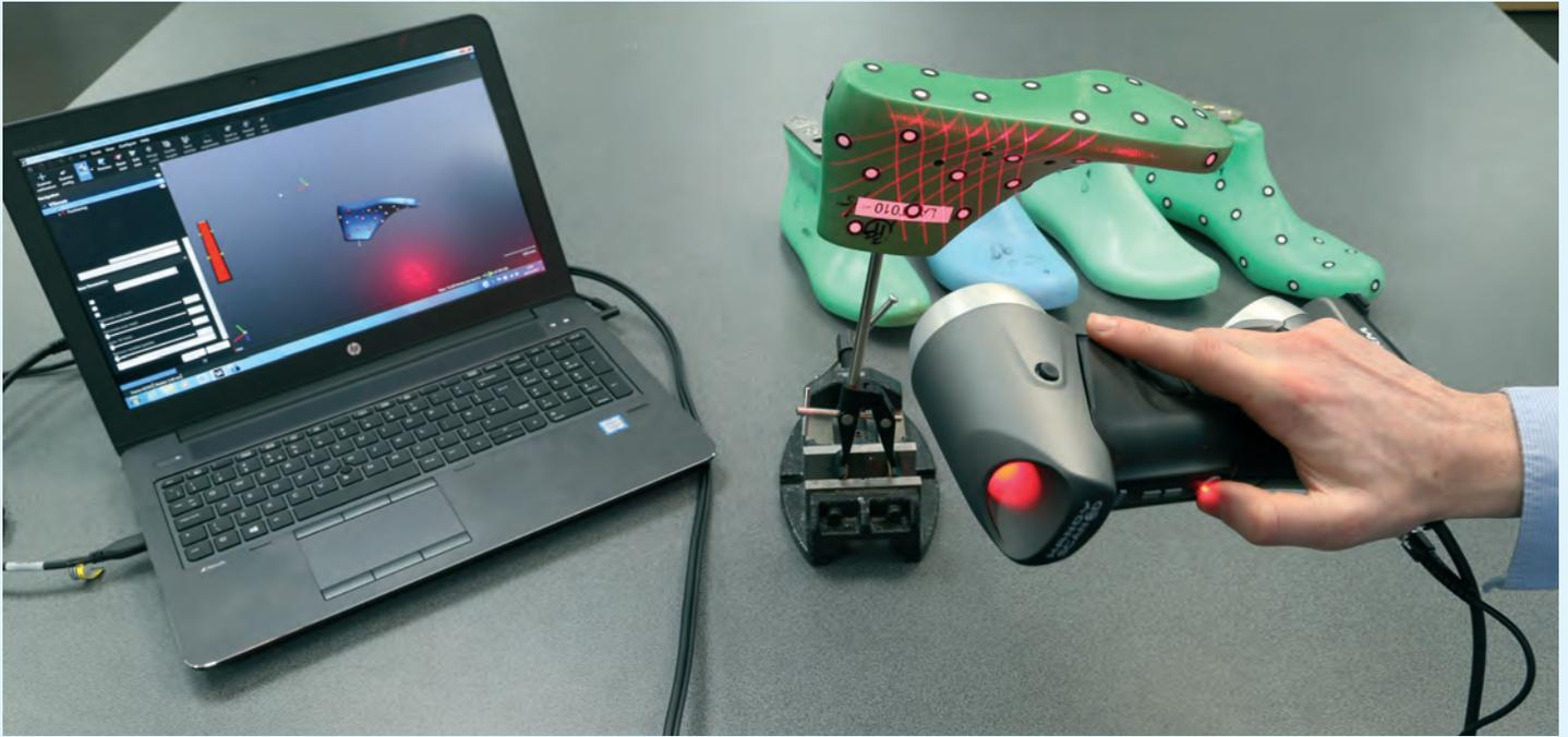
Figure 1: A last being 3D scanned
