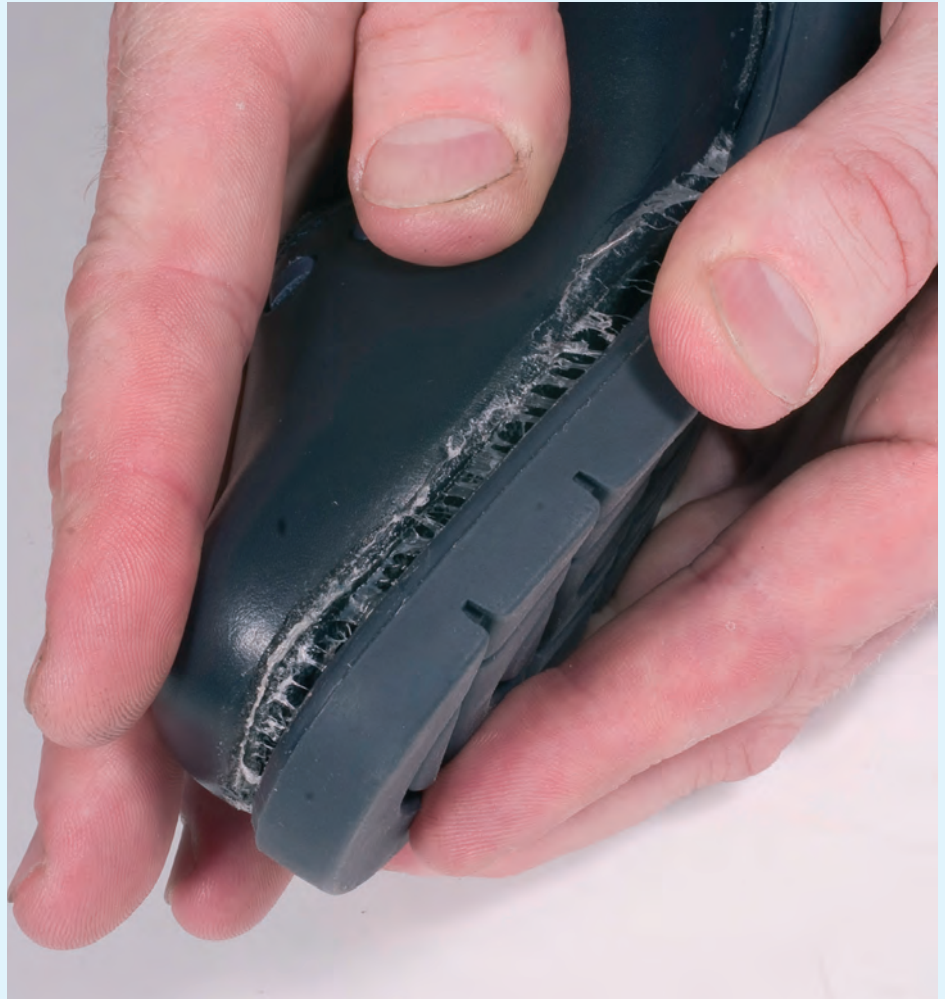
Sole bond failures are a major reason for complaints and, potentially, accidents
