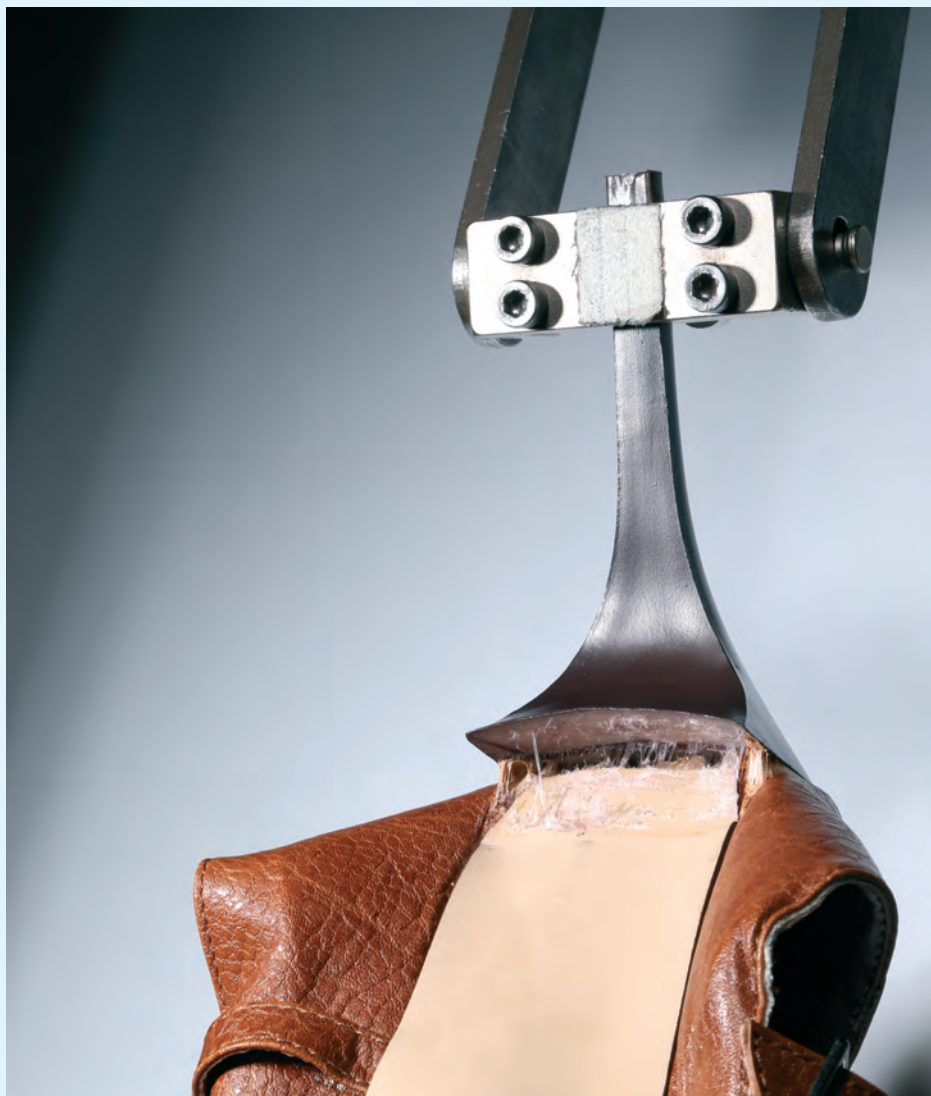
Testing for heel attachment and strength is essential to avoid possible failure during wear
