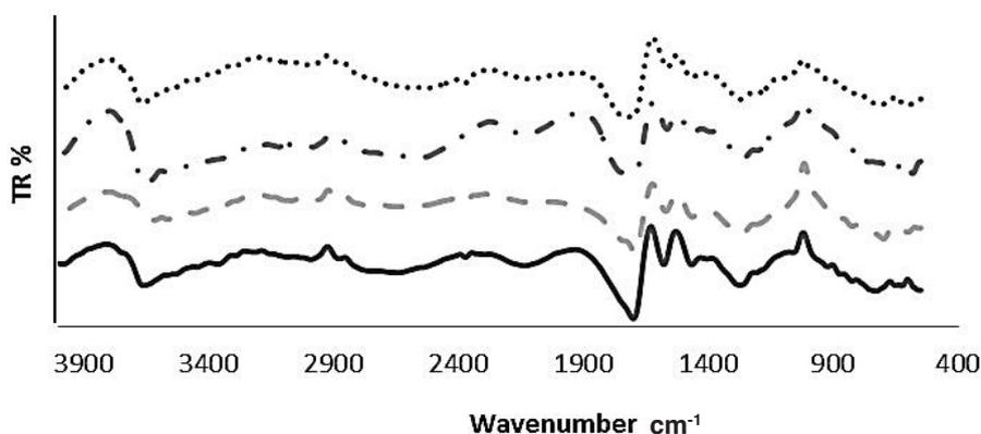
Figure 5. FTIR-ATR spectra of degraded parchment samples inoculated with *T. spectabilis*.
