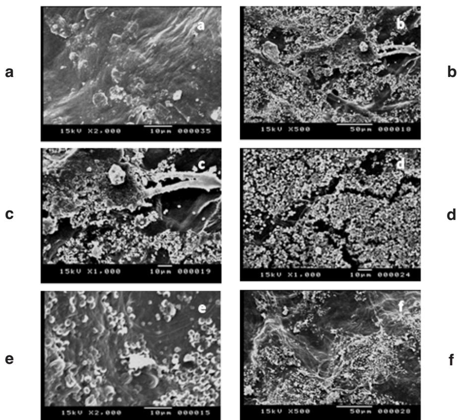
**Figure 6.** a; Fundamental collagen fibres, b; Swollen and rounded fibres, c; Increase of spacing between fibres, d; Loss of fibre network and presence of deep cracks, e-f; Melt-like zones and finally appearance of glassy surface.
