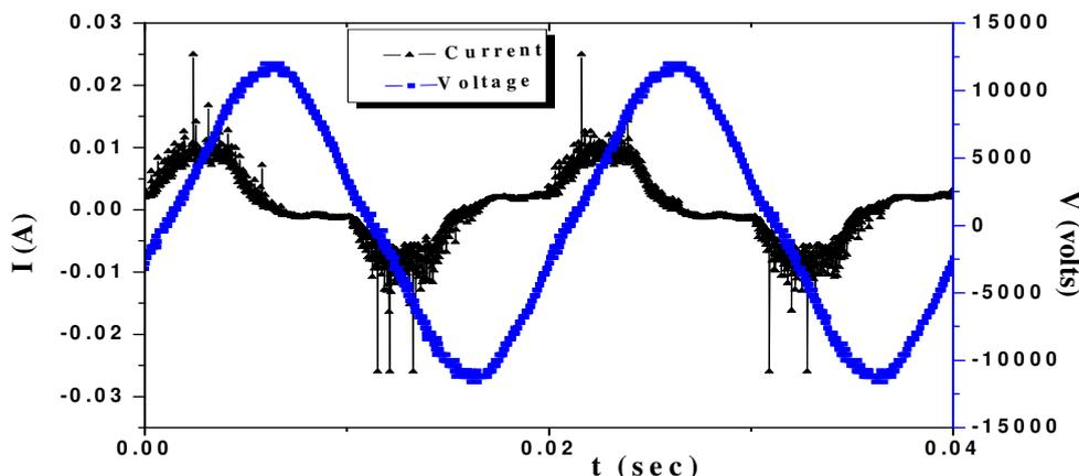
Figure 2. Waveforms of the voltage applied to reactor and associated current.
