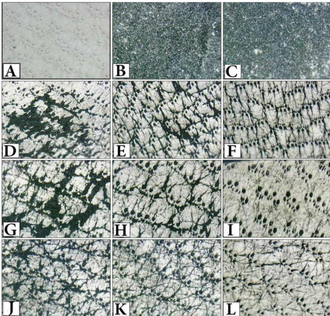
**Figure 5.** Investigation of the surface morphology by digital microscopy: (A) Blank sample, (B) Stained sample, (C) Aged sample, (D~L) Cleaned samples with different powers and time: (D), (E), (F) Cleaned sample with 5.48W after ½, 1 and 2 minutes, respectively, (G), (H), (I) Samples cleaned with 12.21 W after ½, 1 and 2 minutes, respectively, (J), (K), (L) Sample cleaned with 17.35W after ½, 1 and 2 minutes, respectively.
