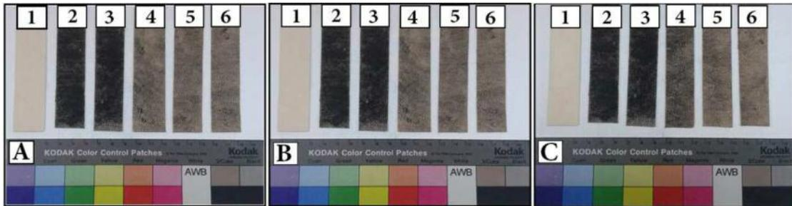
**Figure 4.** Leather samples after plasma cleaning with different powers: (A) Plasma cleaning with 5.48W; (B) Plasma cleaning with 12.21W; (C) Plasma cleaning with 17.35W. The cleaning above was for (1) Blank sample, (2) Stained sample, (3) Aged sample, (4) Cleaned sample after ½ minute, (5) Cleaned sample after 1 minute, (6) Cleaned sample after 2 minutes, respectively.
