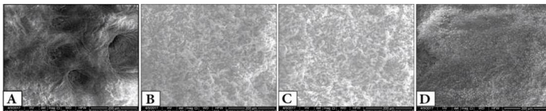
**Figure 6.** Investigation of the surface morphology by SEM: (A) Blank sample, (B) stained sample, (C) Aged sample, (D) Sample cleaned at 17.35W for 2 minutes.
