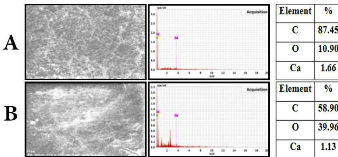
**Figure 7.** EDAX analysis of stained leather before and after plasma cleaning: (A) stained sample before cleaning, (B) stained sample after cleaning.
