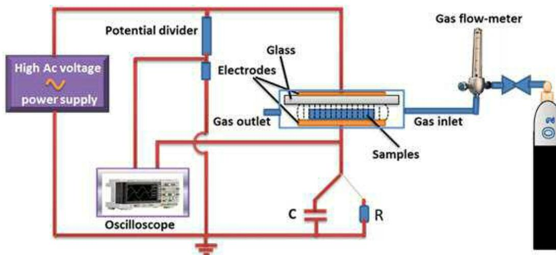
**Figure 1.** The schematic diagram of DBD reactor used in cleaning.
