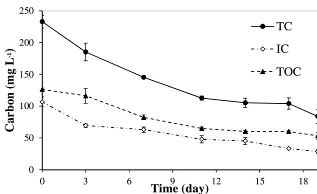
**Figure 7.** Carbon removal along *Tetraselmis sp.* cultivation in composite effluent (75R25T).
