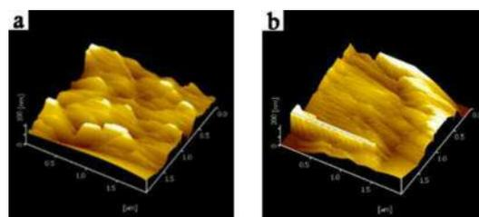
Figure 5. AFM photos of crust leather
