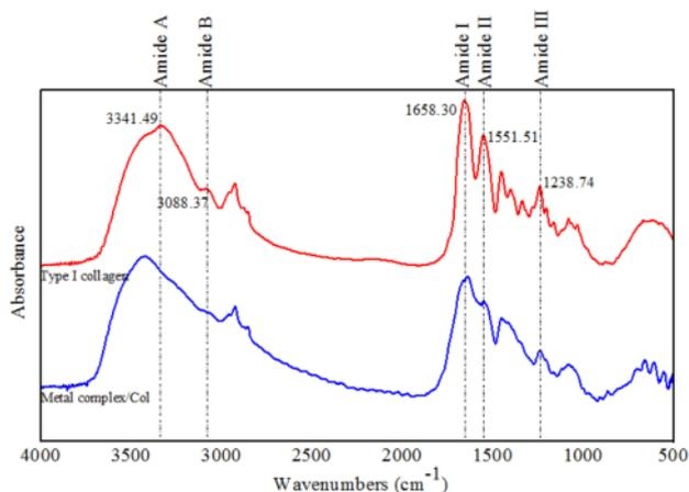
Figure 5. FTIR spectra of Type I collagen treated with Zr-Al-Ti complex.
