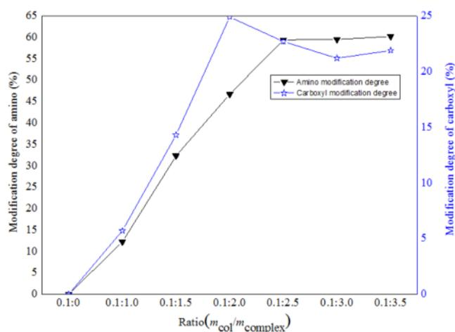
**Figure 4.** Degree of modification of collagen treated by Zr-Al-Ti complex.
