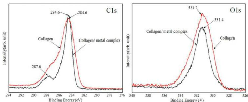
Figure 7. High resolution XPS spectra (a: collagen; b: collagen/metal complex).
