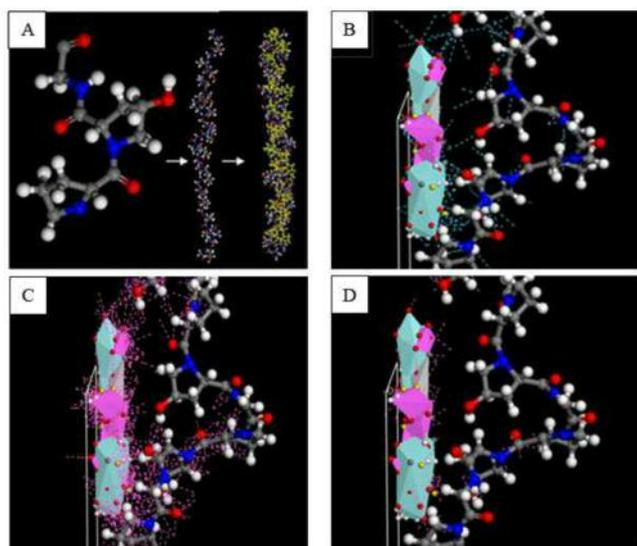
**Figure 3.** Molecular simulation of interactions between collagen and Zr-Al-Ti complex (Gray ball: C, Red ball: O, White ball: H, Blue ball: N; Blue dotted line (B): Hydrogen bond; Pink dotted line (C, D): Close packing).
