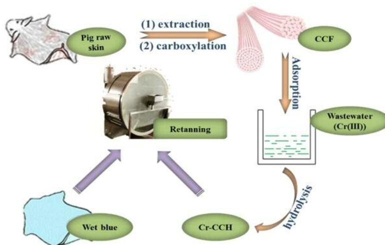
**Scheme 1.** Schematic illustration of the main experimental process
