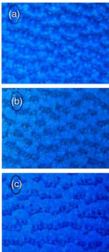
**Figure 5.** Grain of enzymatic treated wet-blue goat leather (a, before ET; b, ET under WBH; c, ET under MIH).
