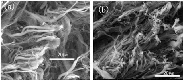
**Figure 2.** SEM images of freeze drying collagen fibres: (a) no retanning and (b) PAA retanning.
