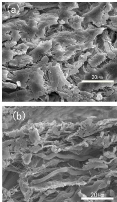
**Figure 3.** SEM images of air drying collagen fibres: (a) no retanning and (b) PAA retanning.
