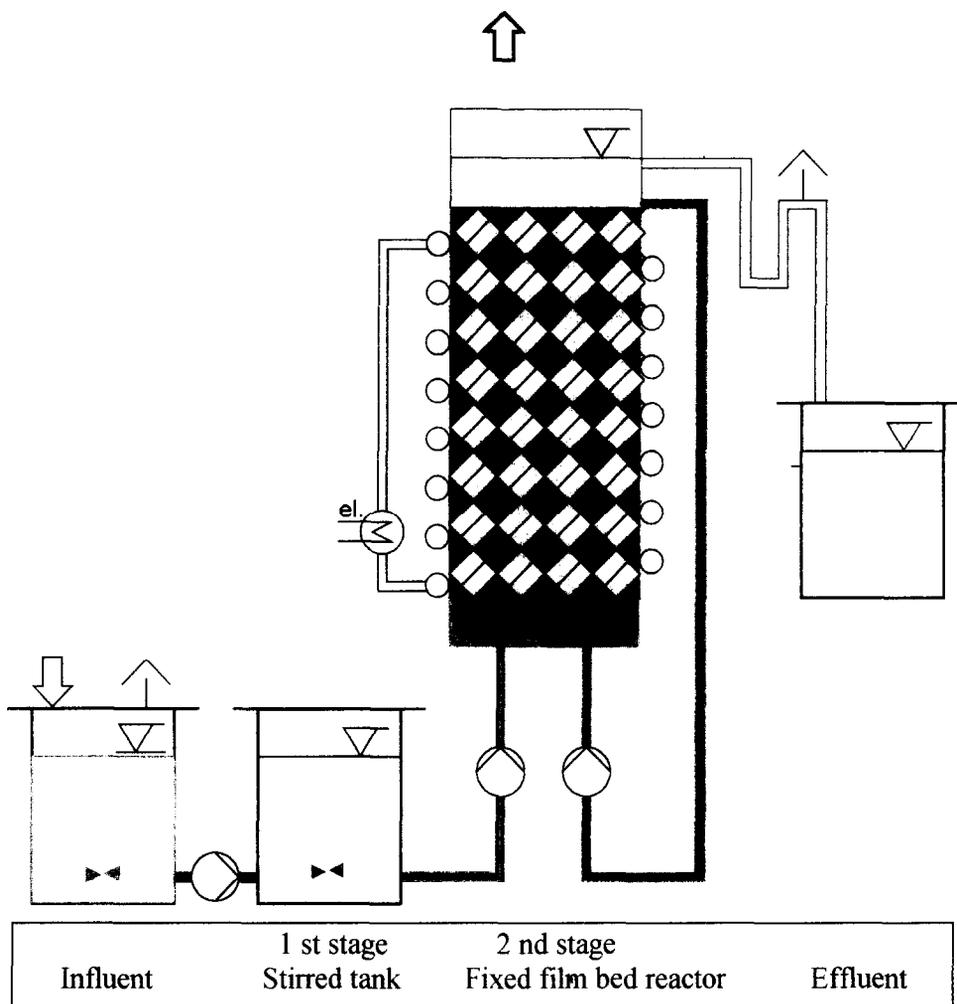
Fig. 1. Treatment scheme of the pilot plant.
