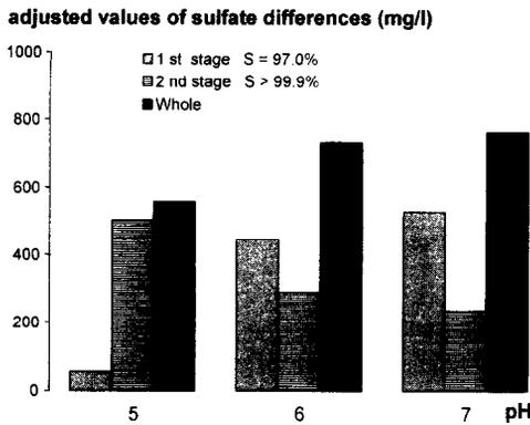
Fig. 5. Influence of pH in the influent on the sulfate differences [ $\text{mg l}^{-1}$ ] (adjusted values, analysis of variance).
