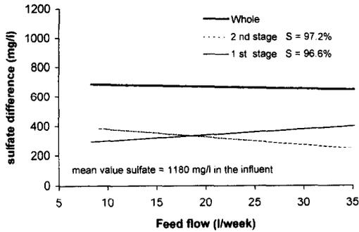
Fig. 2. Influence of feed flow on the sulfate differences [mg l<sup>-1</sup>] (multiple regression).
