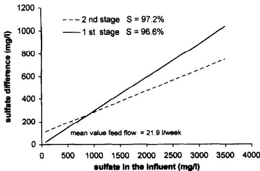
Fig. 3. Influence of sulfate in the influent on the sulfate differences [mg l<sup>-1</sup>] (multiple regression).
