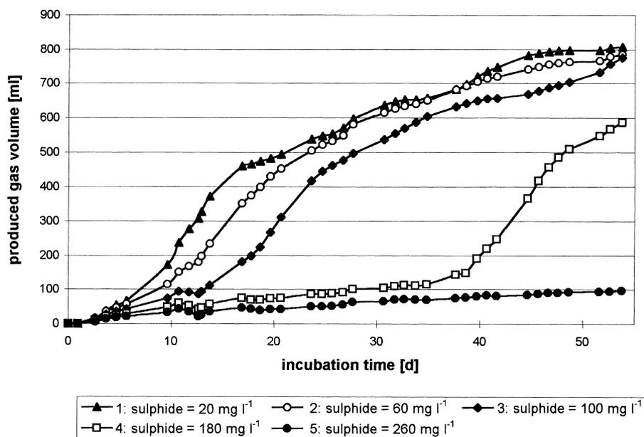
Fig. 2. Temporal development of the produced gas volume in batch experiments with different sulphide concentrations.
