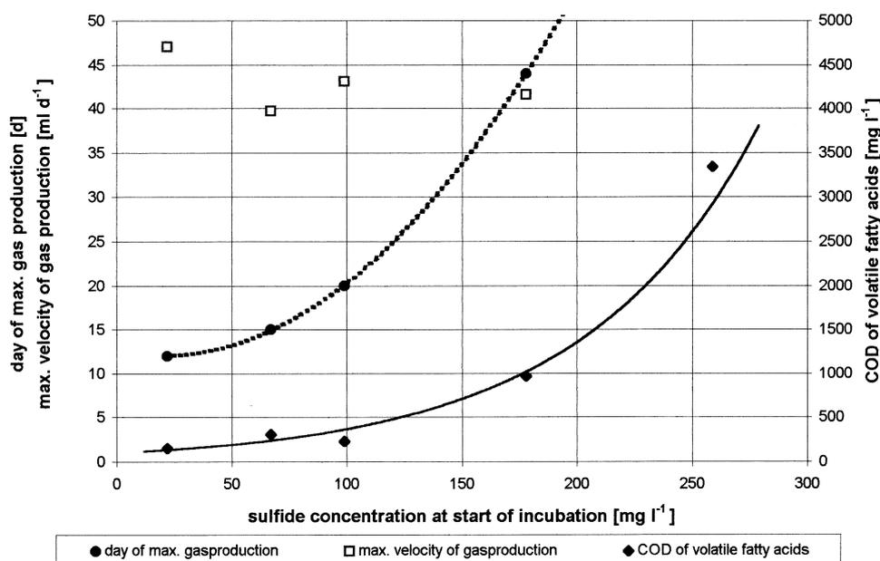
Fig. 3. Day and velocity of maximum gas production and COD of volatile fatty acids correlated with sulphide.
