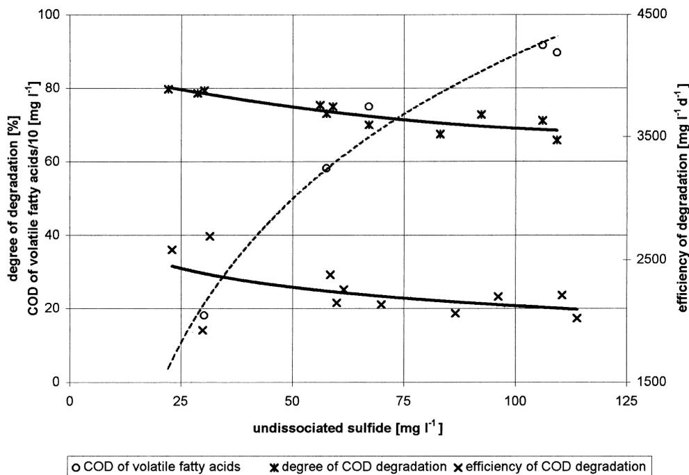
Fig. 4. Reactor 1—degree and efficiency of degradation and COD of fatty acids correlated with undissociated sulphide.
