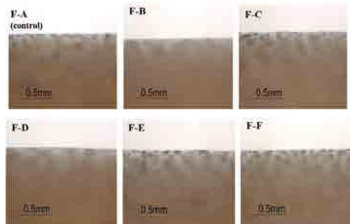
Figure 7. Stereo microscopic images of the leather at the crease made from the differently preserved hides. Bars represent 0.5mm.
