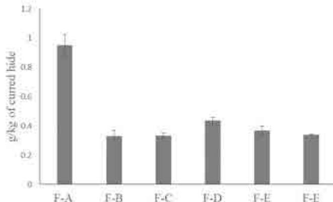
Figure 4. Biochemical Oxygen Demand (BOD) values (in gram) of soaking liquors processing 1 Kg of cured hide.
