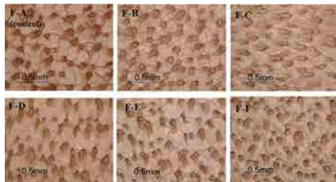
Figure 6. Stereo microscopic images of the leather made from the differently preserved hides. Bars represent 0.5mm.
