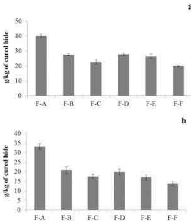
Figure 5. Pollution load generated in the soaking process of hides cured by the different formulations: a) Total Solid (TS) and b) Total Dissolved Solid (TDS)
