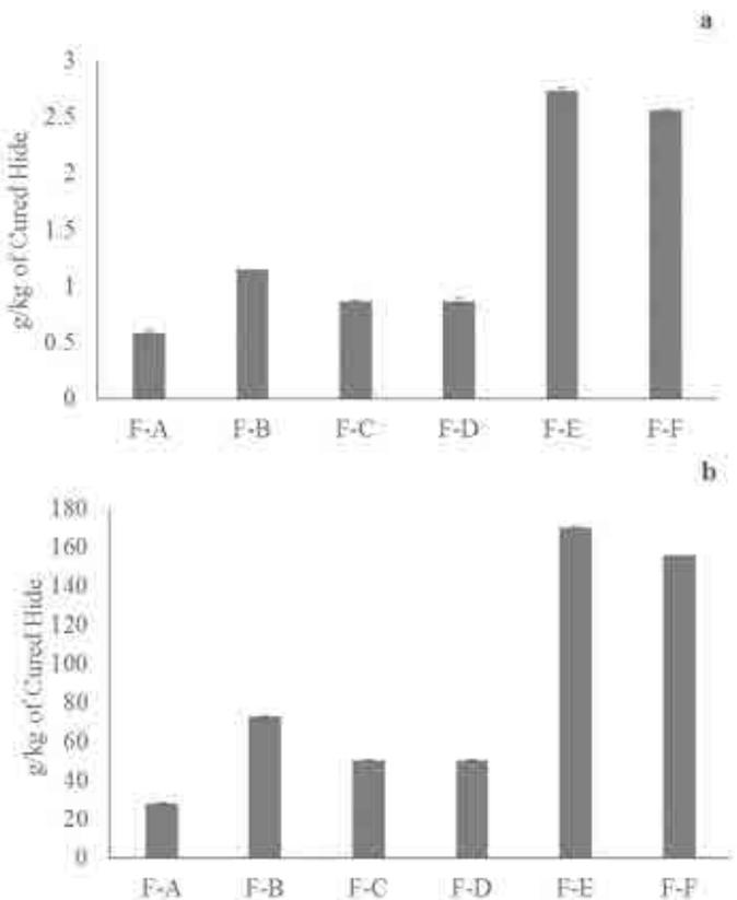
Figure 3. a) Total Organic Carbon (TOC) and b) Chemical Oxygen Demand (COD) values (in gram) of soaking liquors processing 1 Kg of cured hide.
