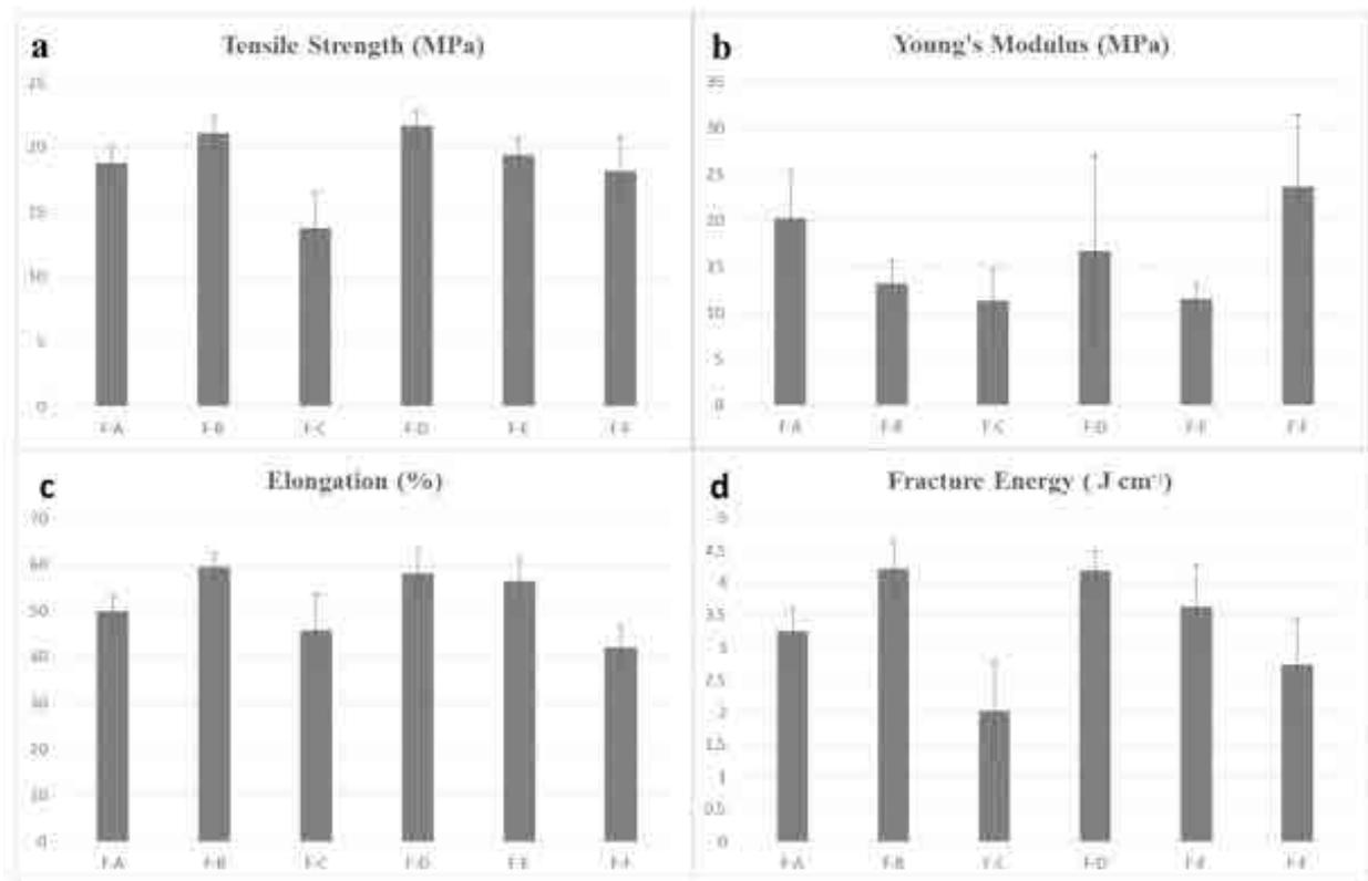
Figure 9. Mechanical properties of the crust upper shoe leather from differently cured bovine hides.
