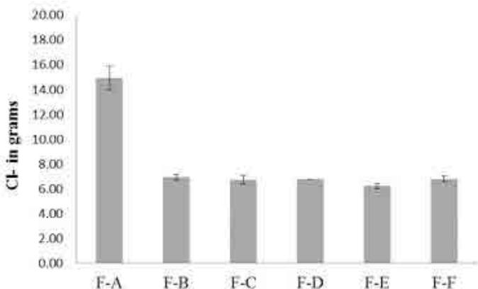
Figure 2. Chloride content of spent liquors generated by soaking of 1 kg of preserved hide
