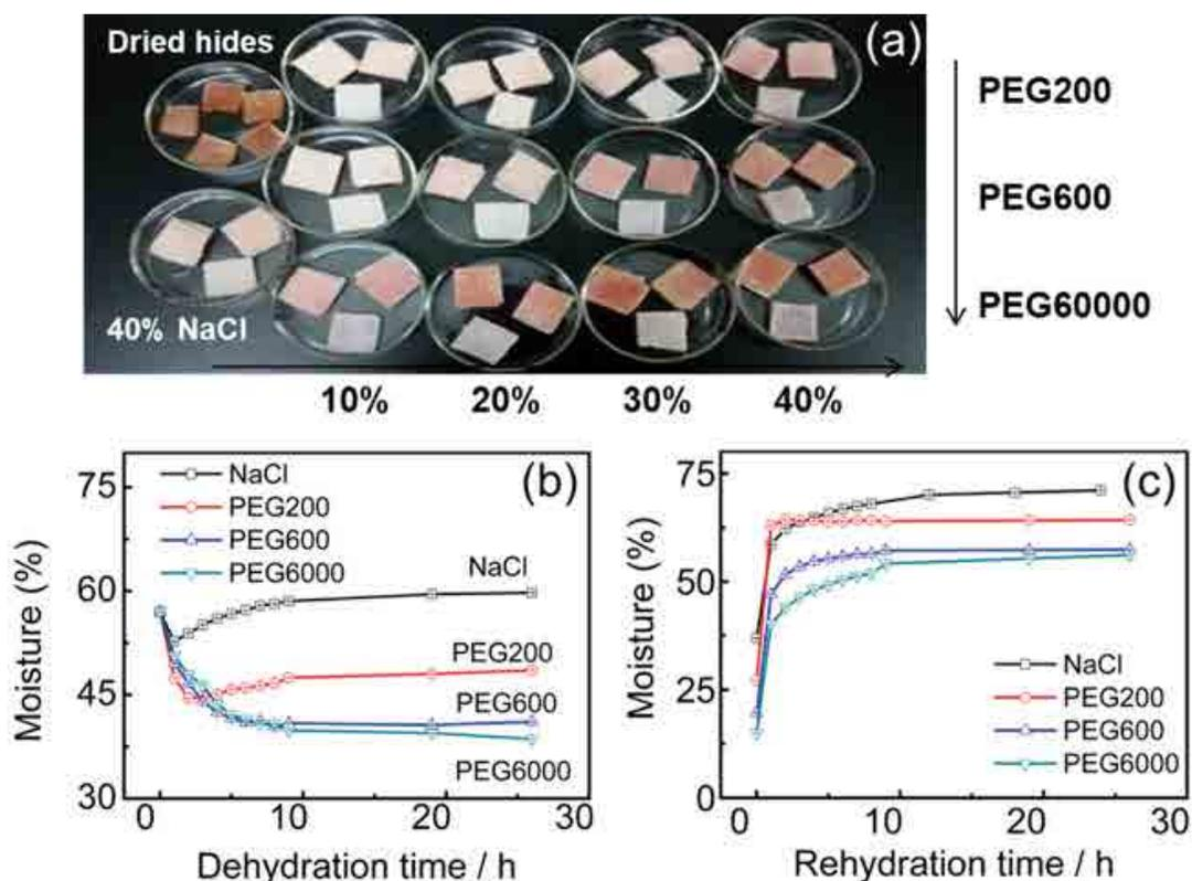
Figure 1. (a) appearance of the preserved samples ( $n=3$ ); (b) time dependence of the moisture contents of the pigskins immersed in 40 wt% of NaCl and PEG with varied  $M_w$ ; (c) rehydration profiles of the preserved pigskins;
