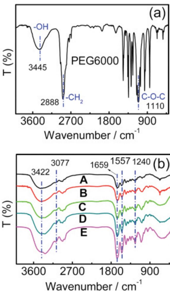
Figure 4. FTIR spectra of (a) PEG and (b) PEG-collagen: (A) collagen, (B) PEG200-Col, (C) PEG600-Col, (D) PEG6000-Col and (E) PEG20000-Col,  $m_{\text{PEG}}/m_{\text{col}} = 20$  wt%.
