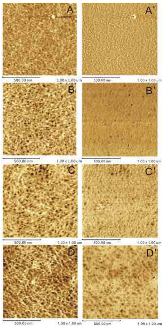
Figure 6. AFM height (left) and phase images (right) of PEG-collagen: (A) collagen; (B) PEG200-Col; (C) PEG4000-Col; (D) PEG6000-Col ( $C_{col} = 6 \times 10^{-6}$  g/mL,  $m_{PEG}/m_{col} = 20$  wt%)
