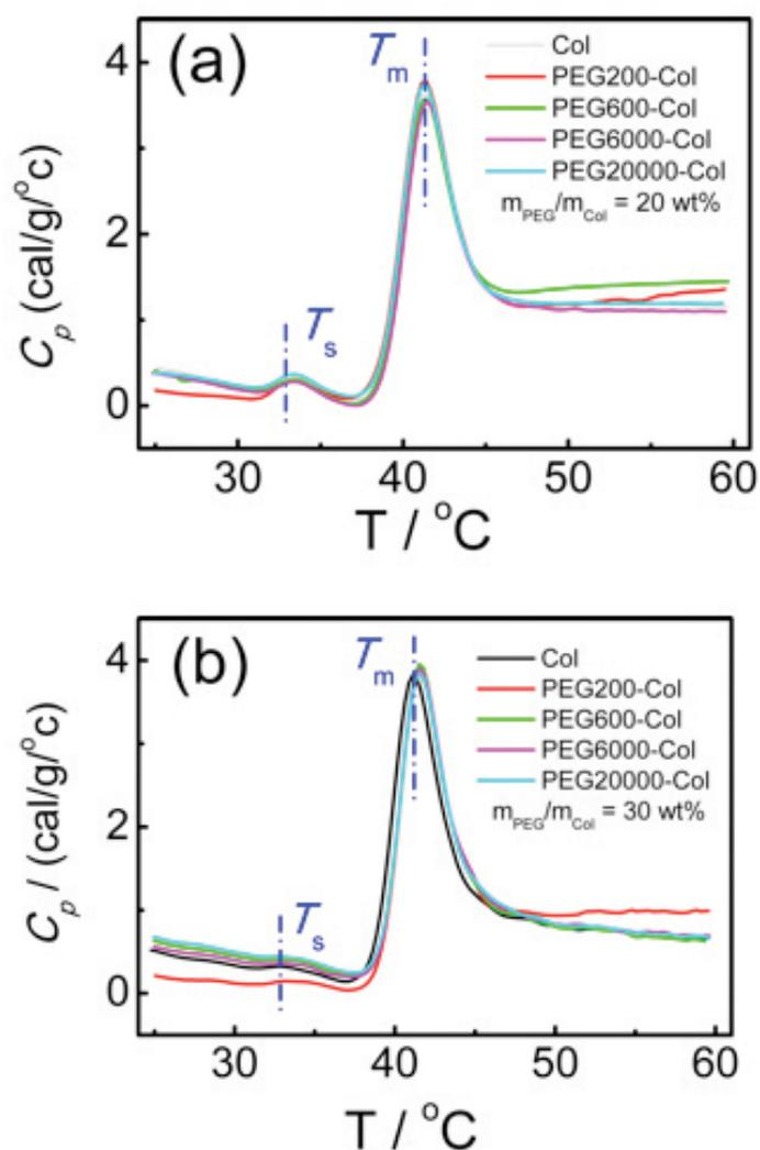
Figure 5. The specific heat capacity ( $C_p$ ) of type I collagen in 0.5 M acetic acid ( $C_{col} = 0.5$  mg/mL) in the presence of PEG with different  $M_w$ : (a)  $m_{PEG}/m_{col} = 20$  wt%; (b)  $m_{PEG}/m_{col} = 30$  wt%.
