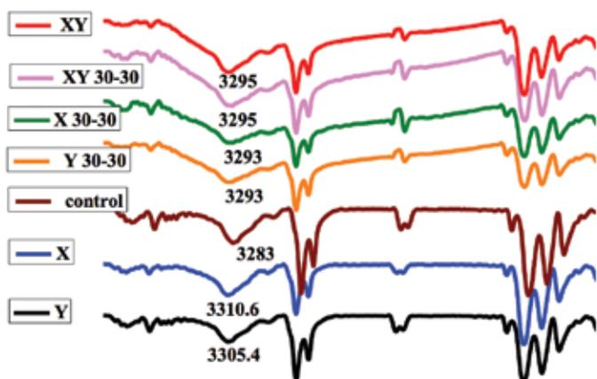
Figure 6. FT-IR spectra of leather experienced different modes of stretching in drying.
