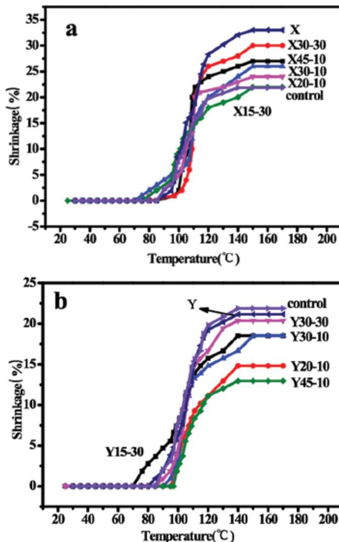
Figure 2. Hydrothermal shrinkage curves of X (a) and Y (b) stretched leather.
