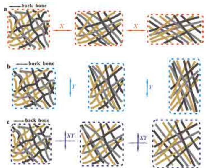
Figure 10. Sketch of fiber orientation in cyclic (a) X stress, (b) Y stress and (c) XY stress.
