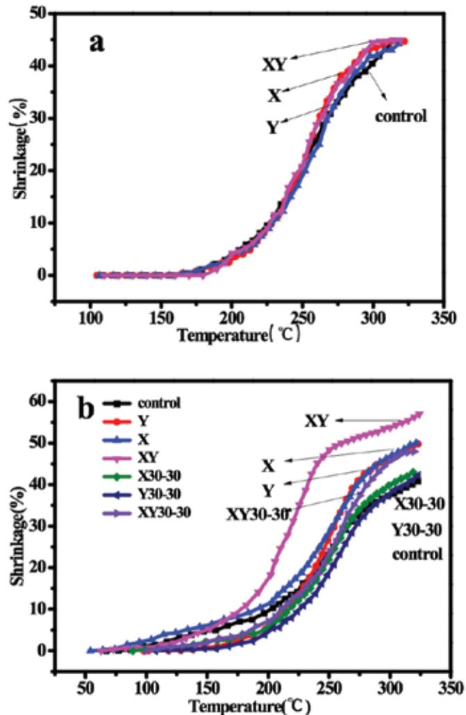
Figure 4. Dry heat shrinkage curves of (a) XY stretched collagen fiber and (b) leather sheet.
