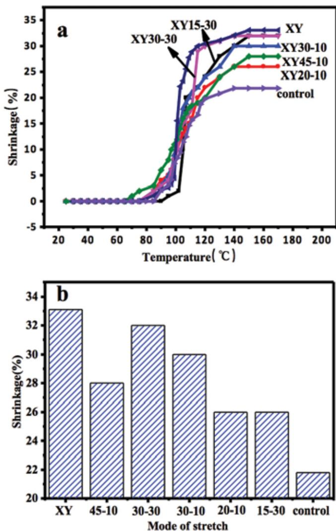
Figure 3. (a) Hydrothermal shrinkage curves and (b) shrinkage ratio of XY stretched leather.
