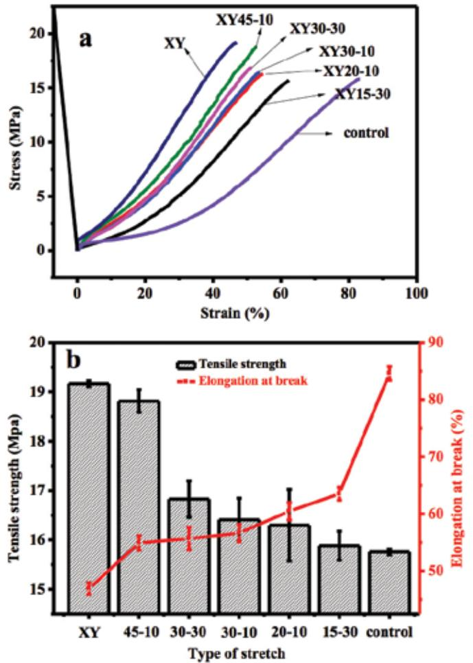
Figure 9. (a) Stress-strain curves, (b) tensile strength and elongation of XY stretched leathers.
