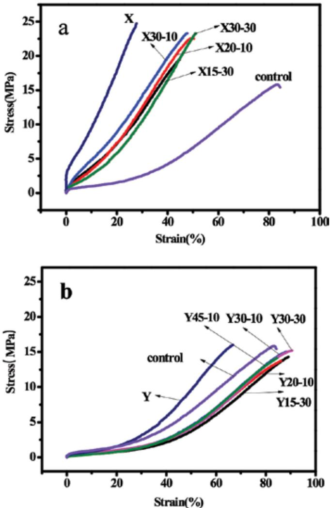
Figure 8. Stress-strain curves of (a) X and (b) Y stretched leather.
