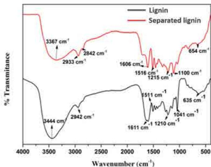
Figure 1. FT-IR Spectrum of the separated and standard lignin.
