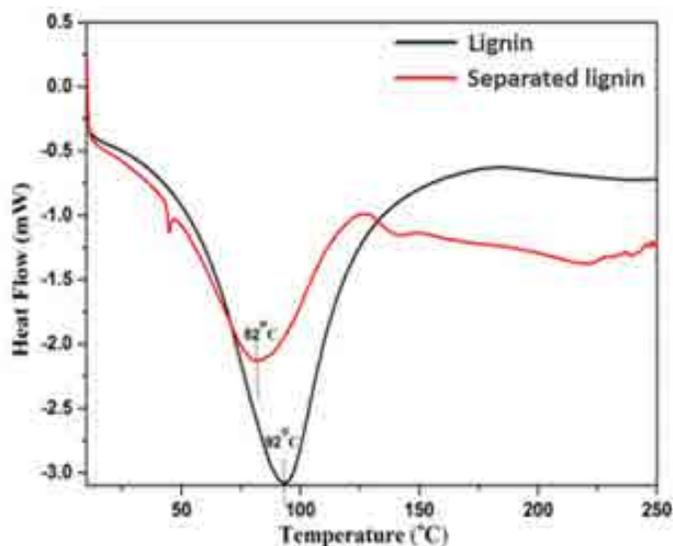
Figure 3. Differential Scanning Calorimetric profile of the separated and standard lignin.
