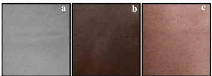
Figure 6. Surface color of the leather a) uncoated, b) coated with lignin based pigment formulation, and c) commercial brown pigment.
