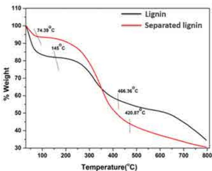
Figure 2. TGA curve of the separated and standard lignin.
