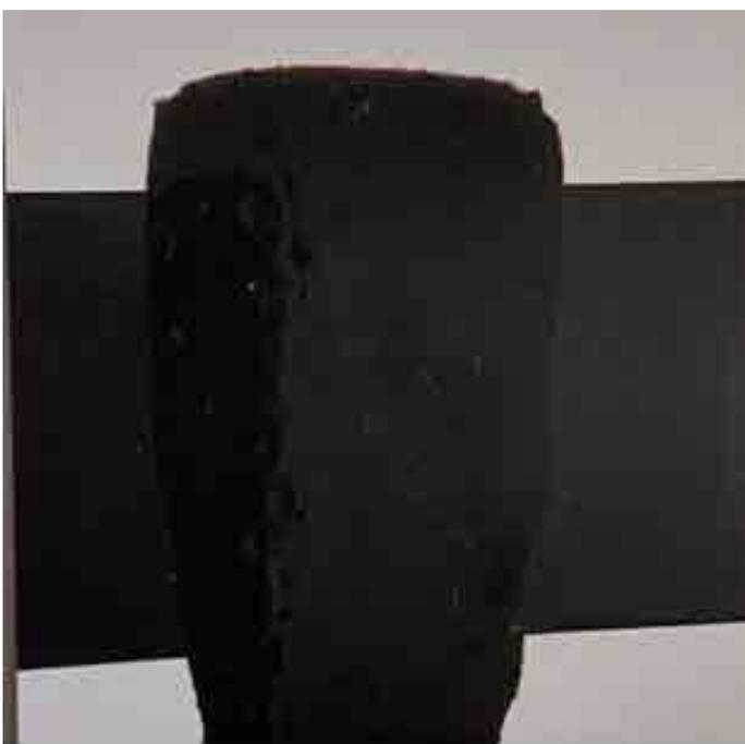
Figure 5. Mass tone/hiding power of the lignin based pigment coated checkered card.
