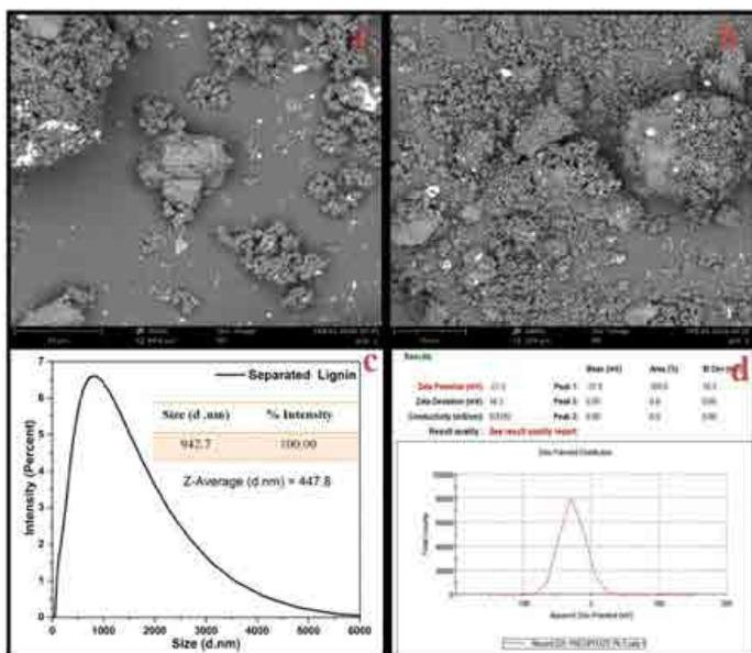
Figure 4. Scanning Electron Microscopic images (a, b), hydrodynamic diameter (c) and their corresponding surface potential (d) of lignin based pigment.
