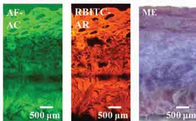
Figure 4. Fluorescence micrographs (green and red) and photomicrographs (brown) of vertical sections of the retanned leathers. (a) retanning with 3% AF-AC, 3% RBITC-AR or 3% ME for 90 min, (b) retanning with 3% AF-AC for 30 min, then with 3% RBITC-AR and 3% ME for 60 min.
