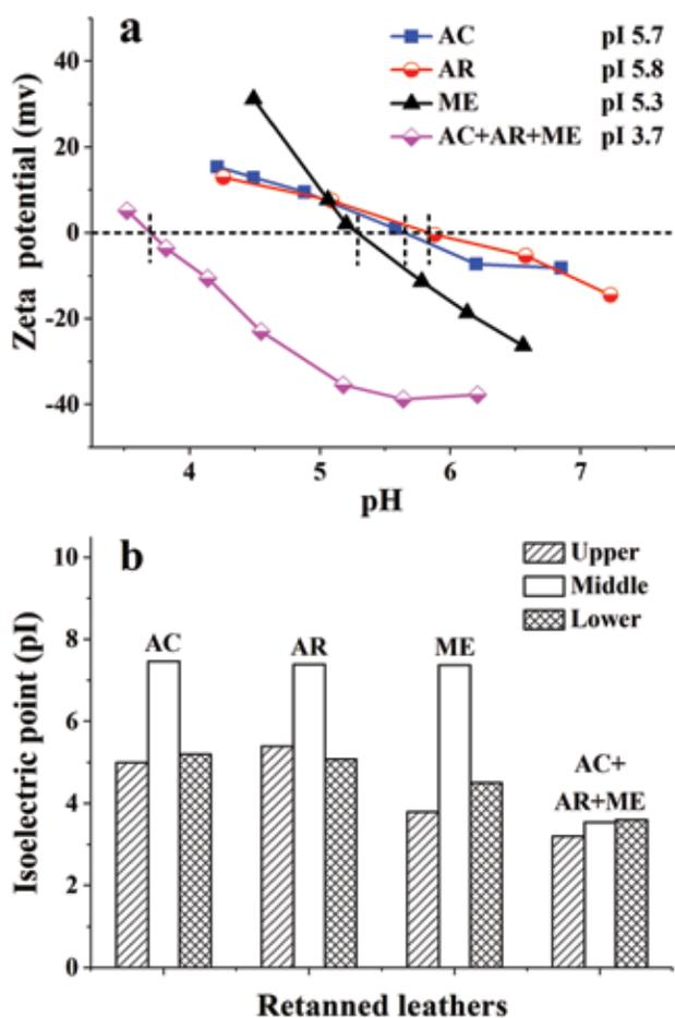
Figure 3. Isoelectric points (pIs) of the retanned leathers (a) and pIs of each layer of the retanned leathers (b).
