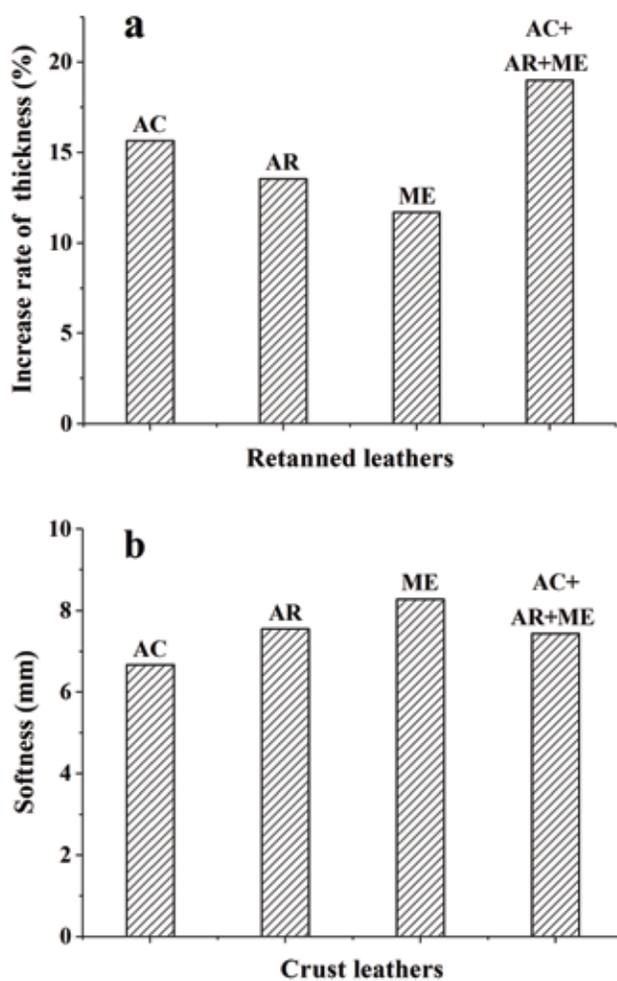
Figure 7. Thickness increase rate of the retanned leathers (a) and softness of the crust leathers (b).
