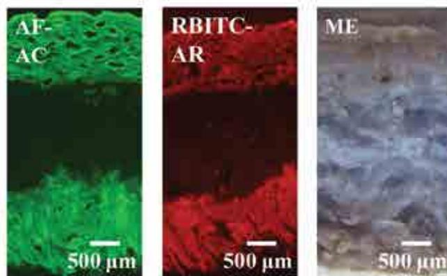
**b Retanning with 3% AF-AC for 30 min, then with 3% RBITC-AR and 3% ME for 60 min.**
