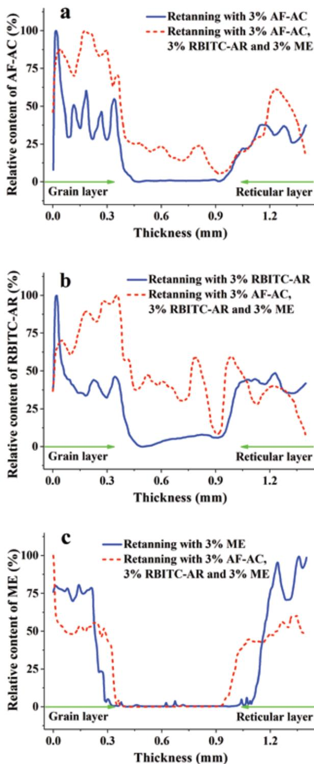
Figure 5. Relative contents of AF-AC (a), RBITC-AR (b) and ME (c) in the retanned leathers that were semi-quantified by analysis of Figure 4 using Image J software.
