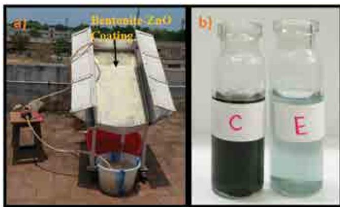
Figure 6. The photograph of the a) solar photoreactor used for degradation of post tanning wastewater using semiconductive Bentonite-ZnO mixed oxide catalyst and b) Visual assessment of colour change during before (C) and after (E) catalytic treatment.
