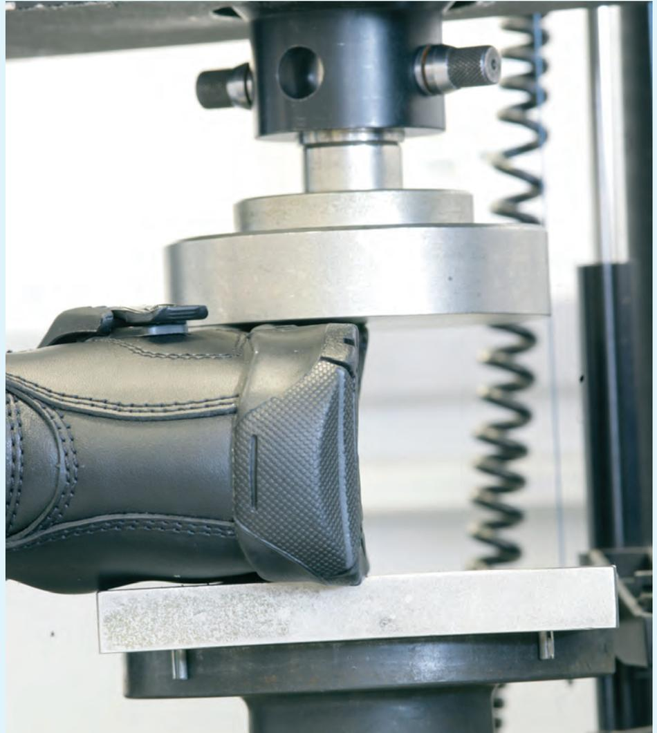
Figure 3: The transverse rigidity test
