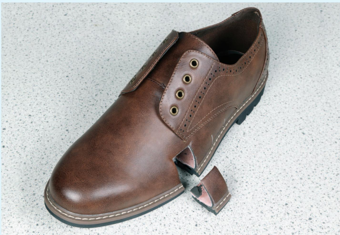
*A peel strength specimen cut from the sole bond of a finished shoe*
