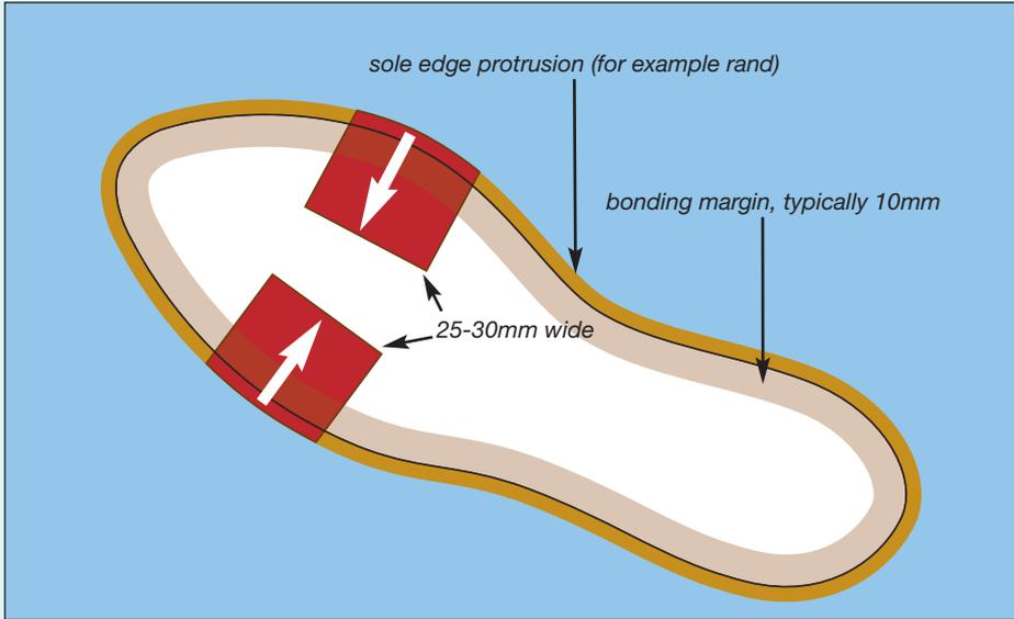
Figure 2: Sections are cut from the flexing joints. White arrows show direction of peel
