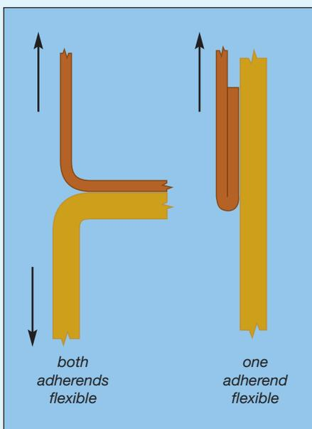
Figure 1a: Sole adhesion peel strength tests are made at 180 degrees, requiring flexibility of at least one adherend
