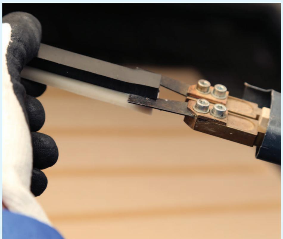
Figure 6: Preparing a specimen with a heated metal blade
