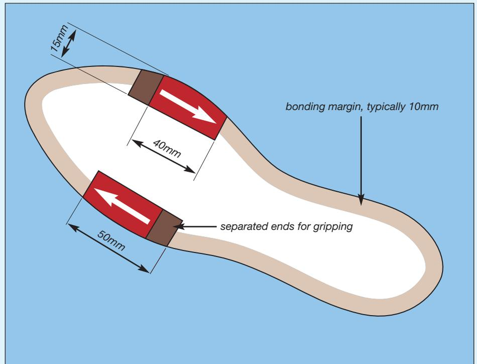
Figure 5: Sections are cut from reasonably straight areas close to the flexing joints. Arrows show the direction of peel, which may be forwards or backwards
