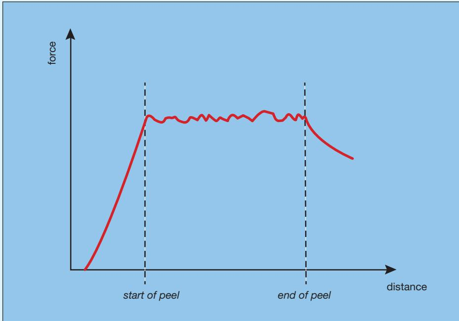
Figure 7: Typical 'along' peel trace shape
