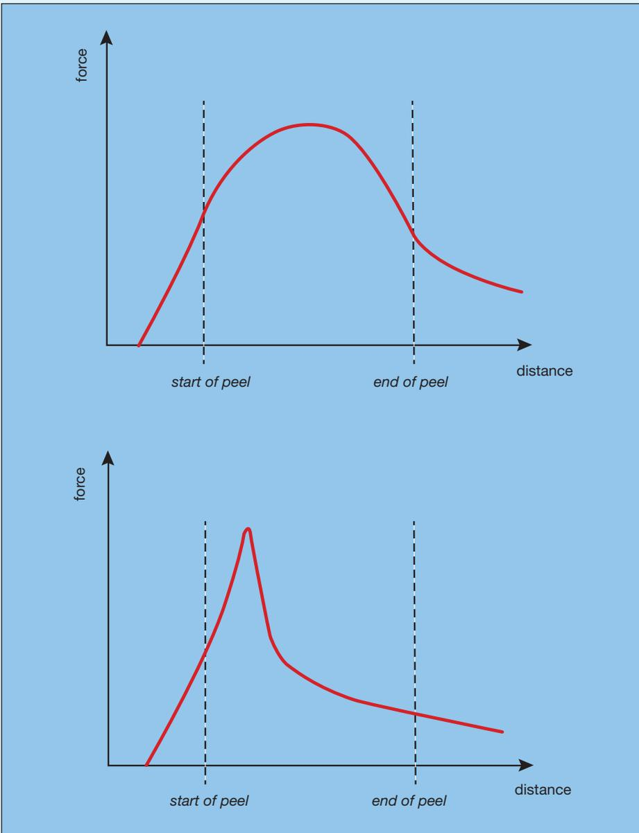
Figure 3: Typical 'across' peel trace shapes
