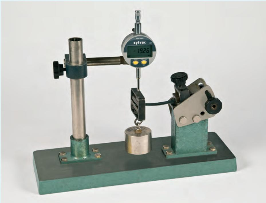
Figure 2: Measuring the stiffness of a shank
