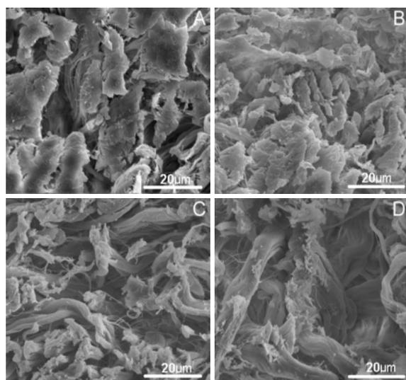
Figure 4. SEM images of collagen fibres retanned with different PAA dosages. (A) 0, (B) 3%, (C) 6%, (D) 9%.
