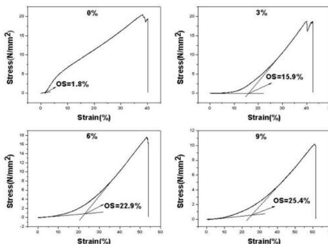
Figure 5. Strain-stress curves of leather retanned with different PAA dosages.
