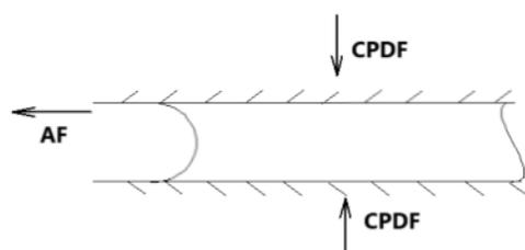
Figure 3. Stress state sketch map of capillary wall after PAA retanning.
