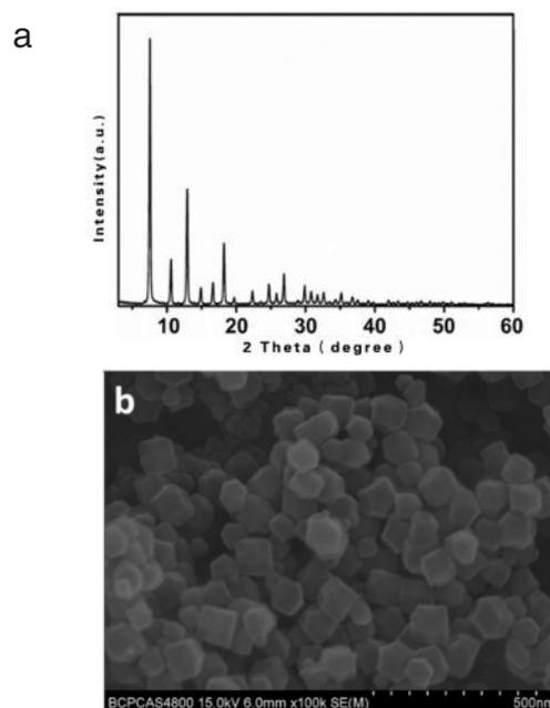
Figure 1. XRD (a) and SEM (b) of ZIF-8 samples.
