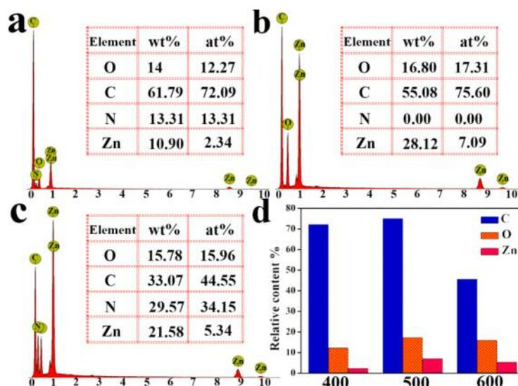
Figure 6. (a-c) shows EDS element analysis in Z400, Z500 and Z600, and (d) shows the relative content of each element
