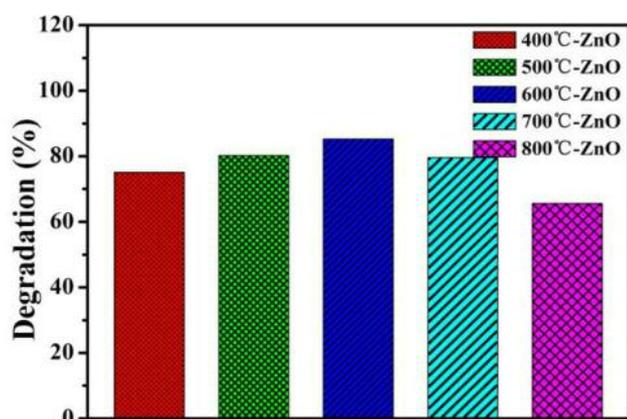
Figure 10. COD removal rate of dyeing wastewater degraded by Z400-Z800.
