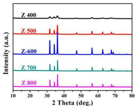
**Figure 3.** X-ray diffraction patterns of Z400-Z800.
