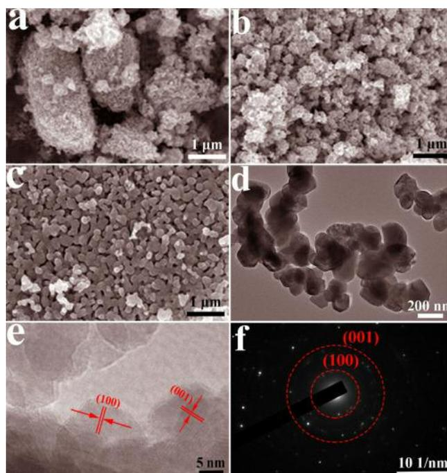
**Figure 4.** (a-c) SEM of Z400, Z500, Z600, TEM of (d) Z600, (e) lattice fringe, (f) crystal diffraction ring.
