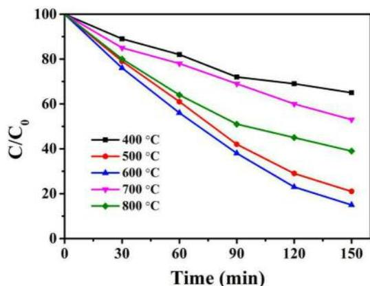
Figure 8.  $C/C_0$  curve of photocatalytic degradation of MB by ZnO prepared at different calcination temperatures over time.
