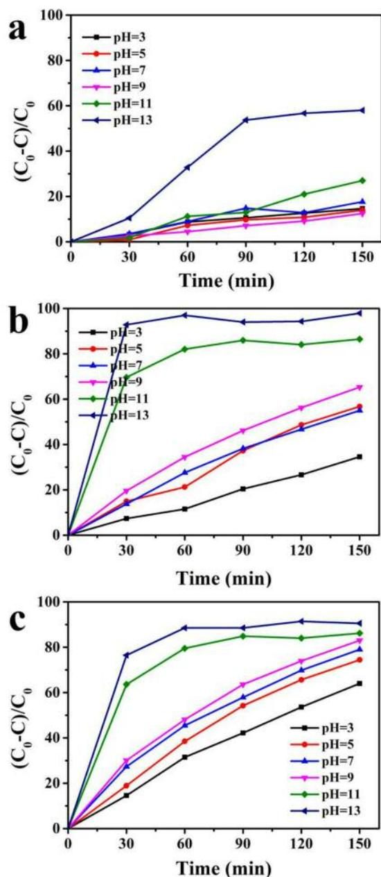
Figure 9. Degradation rates of Z400, Z500 and Z600 for photocatalytic degradation of MB over time under different pH conditions.
