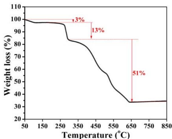
Figure 2. Thermogravimetric curve of ZIF-8.
