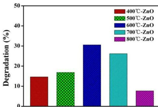
Figure 11. Z400-Z800 degradation of dyeing wastewater TOC mineralisation rate.
