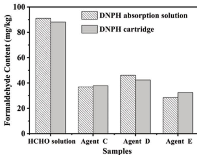
Figure 6. Effect of derivative devices on the determination of formaldehyde.
