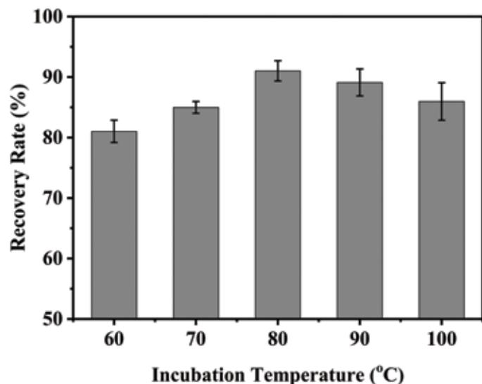
Figure 3. The effect of incubation temperature on the recovery rate of formaldehyde.
