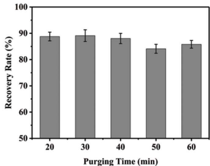
Figure 4. The effect of purging time on the recovery rate of formaldehyde.
