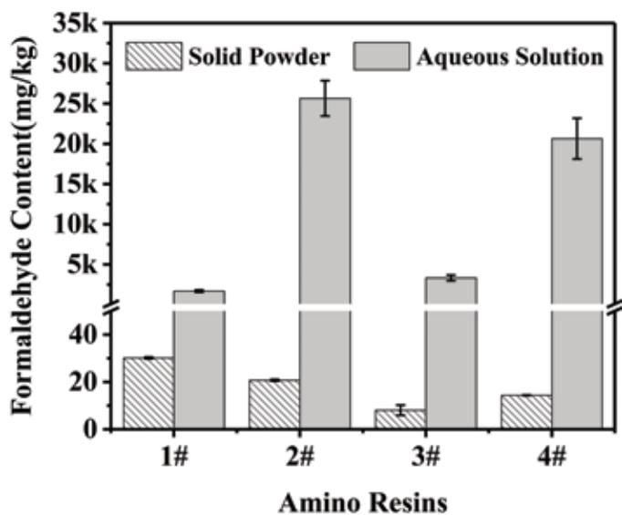
Figure 7. Formaldehyde content in powdery amino resins and their aqueous solutions.
