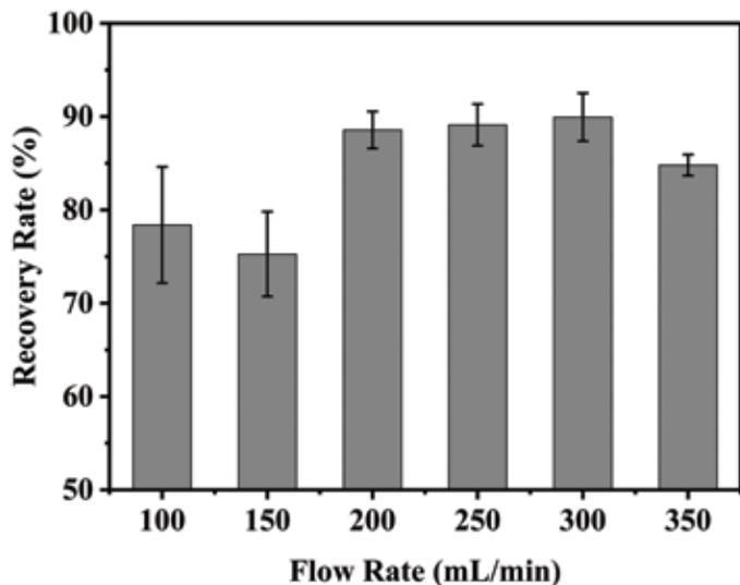
Figure 2. The effect of nitrogen flow rate on the recovery rate of formaldehyde.
