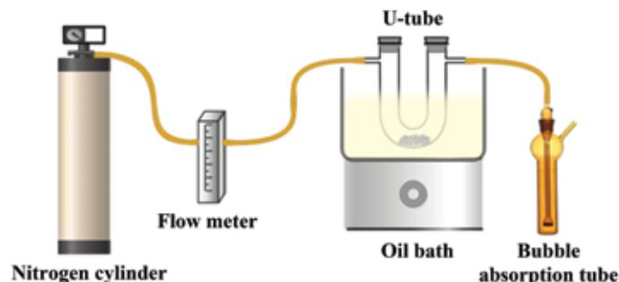
Figure 1. Schematic diagram of the formaldehyde extraction system.
