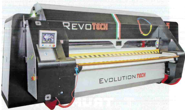
Revotech Rotary press – incorporating patented technology to improve print capability and reduce pressure and temperature.
