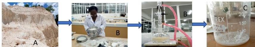
**Figure 1.** Step by step preparation of aluminium sulphate from Pugu kaolin (A=Kaolin deposit, B=Preparation and extraction, C=Aluminium sulphate)
