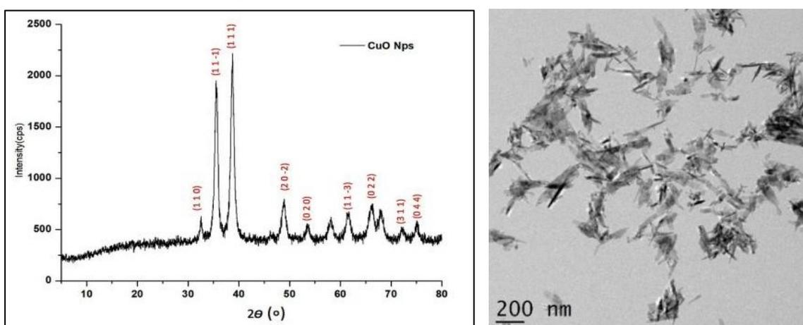
Fig. 1. XRD and TEM of synthesized CuO Nps
