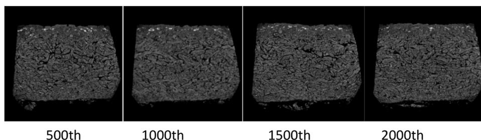
**Figure 3.** Leather section images reconstructed from the series CT projection images.
