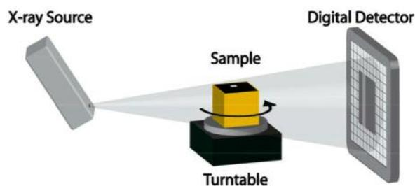
Figure 1. Schematic diagram of micro-CT system.
