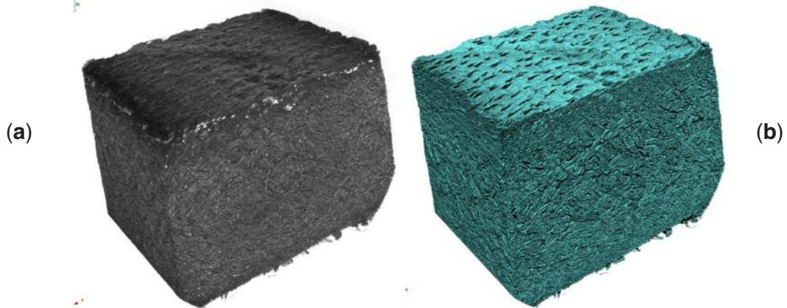
**Figure 5.** 3D volume rendering reconstruction images of leather (5.4mm × 3.5mm × 3.9mm).
