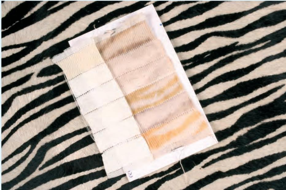
Figure 2: Testing colour fastness to water. In this example, the black zebra stripes have heavily stained the SATRA test material – a characteristic which would likely lead to complaints
