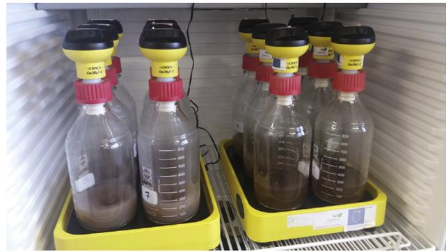
Fig. 1. The OxiTop<sup>®</sup> system operating in an incubation chamber, including pressure sensors, flasks, and stirring plates.
