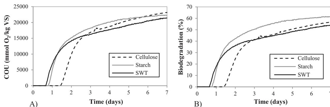
**Fig. 2.** Evaluation of the cumulative oxygen uptake (COU) (A) and biodegradation levels (B) of cellulose, starch, and SWT over a 7-day test period. In each case, the results were calculated as mean values of six replicates.
