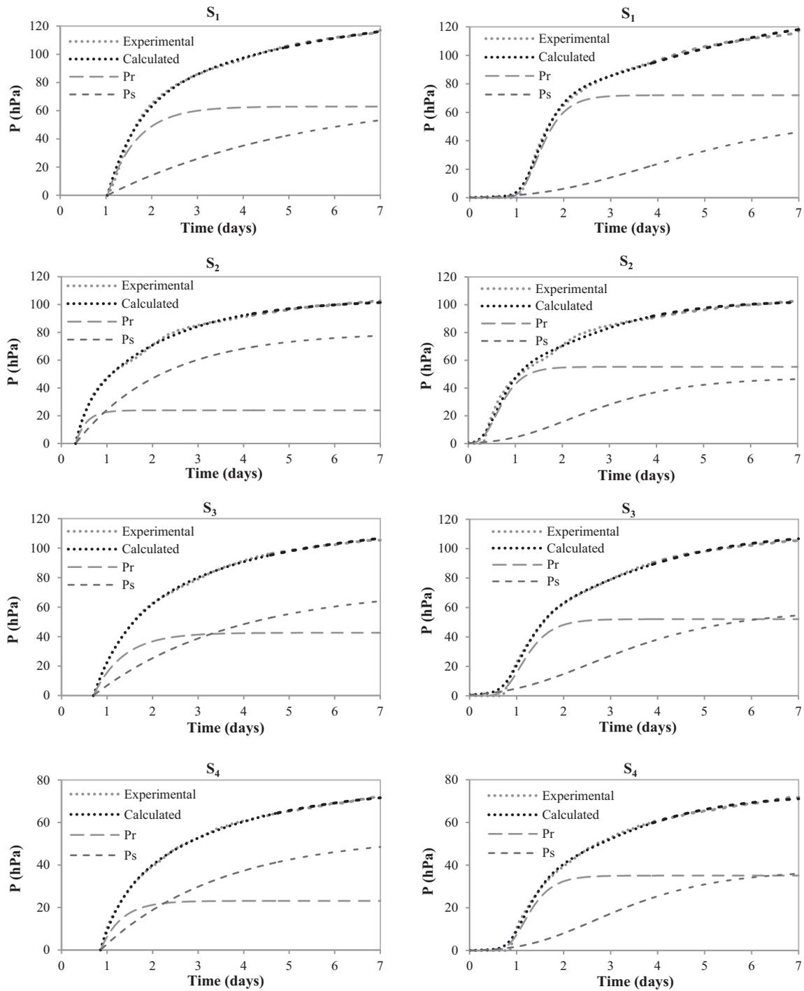
**Fig. 4.** OxiTop® pressure-evolution data for leather samples fitted with the double exponential (left) and Gompertz (right) models. Pr and Ps represent the modelled curves for rapidly and slowly degradable substrates, respectively.
