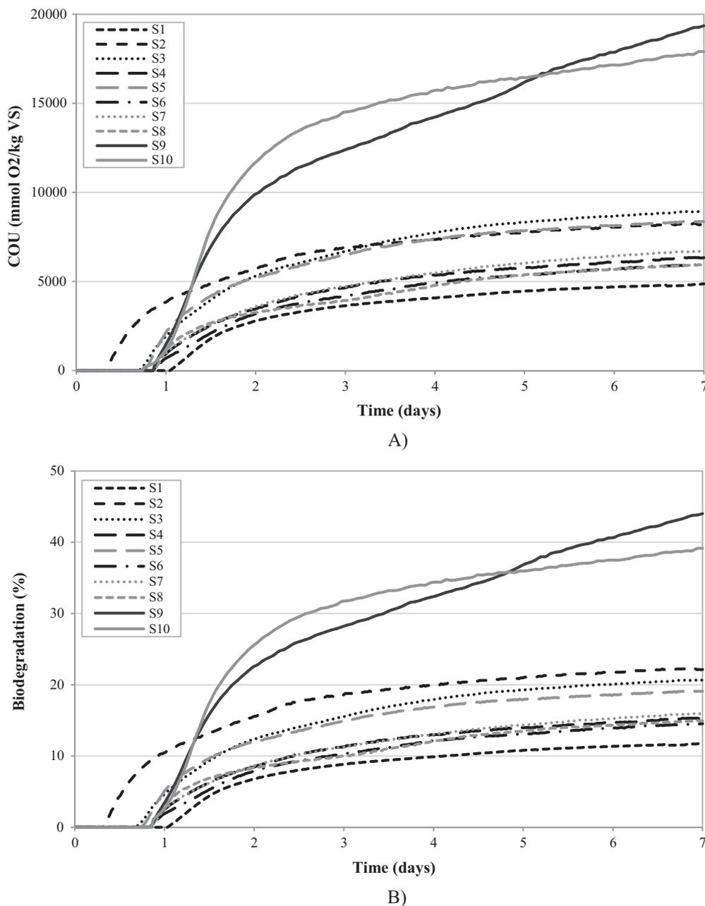
Fig. 3. Evolution of the cumulative oxygen uptake (COU) (A) and biodegradation (B) of different leather materials over the 7-day test period. In each case, the results were obtained as mean values of a set of replicates: four replicates (S<sub>5</sub> and S<sub>10</sub>), five replicates (S<sub>2</sub>, S<sub>3</sub>, S<sub>4</sub>, S<sub>7</sub>, and S<sub>8</sub>), and six replicates (S<sub>1</sub>, S<sub>6</sub>, and S<sub>9</sub>).
