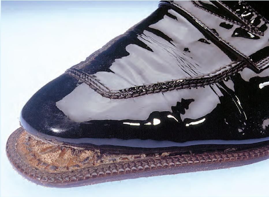
Figure 1: SATRA has seen a number of cases where the wearer has tripped because a sole became loose
