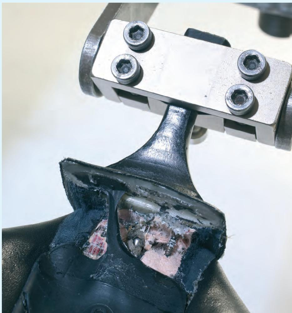
Figure 2: Assessing heel attachment strength
