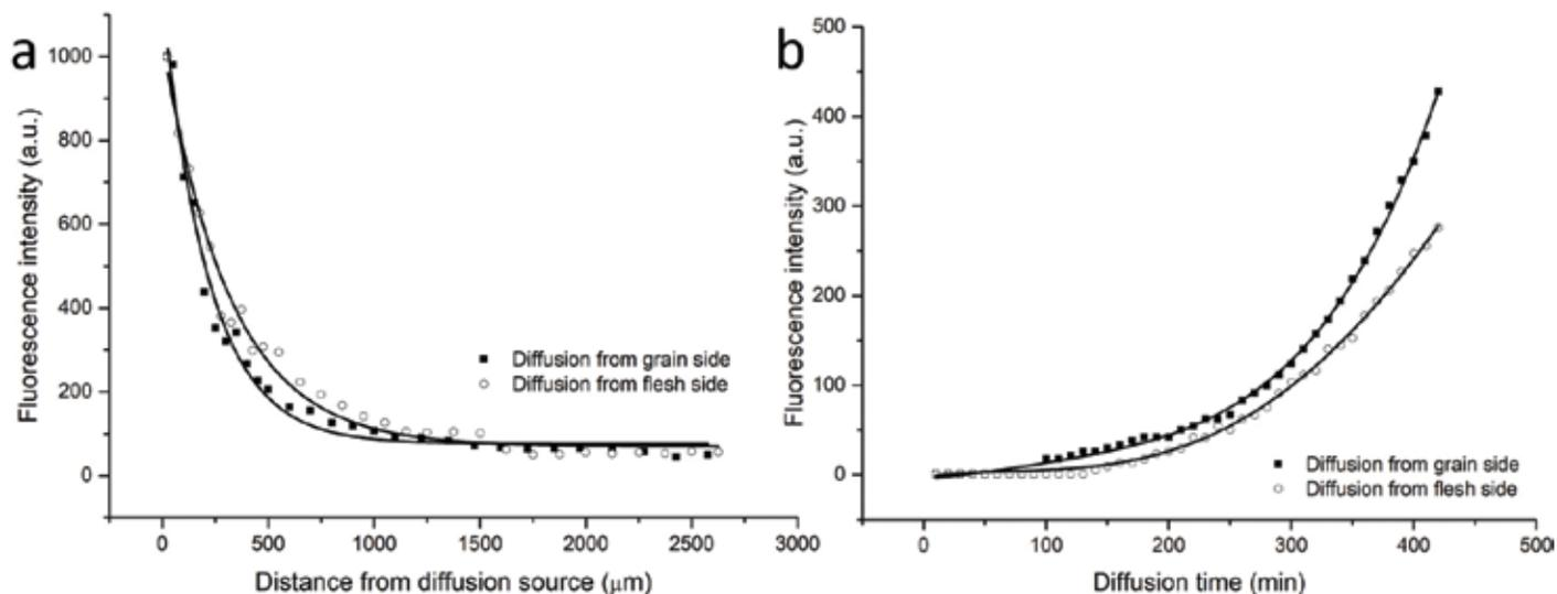
Figure 4. (a) Distribution of FITC-trypsin in goatskin matrix processed for 15 min. (b) Dependence of fluorescence intensity of buffer solution on diffusion time.
