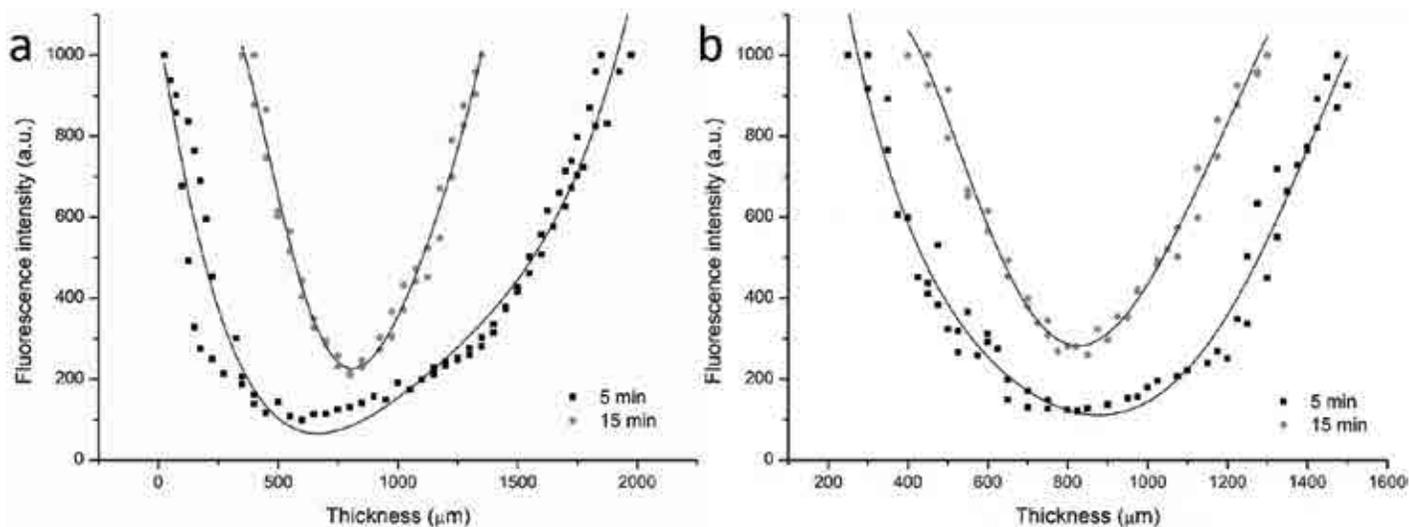
Figure 5. Fluorescence intensity in different portions of goatskin with turbulent diffusion. (a) Back area; (b) Belly area.
