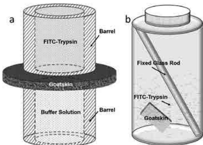
Figure 1. Designed apparatus for enzyme diffusion evaluation (a) in one-way diffusion and (b) turbulent diffusion.
