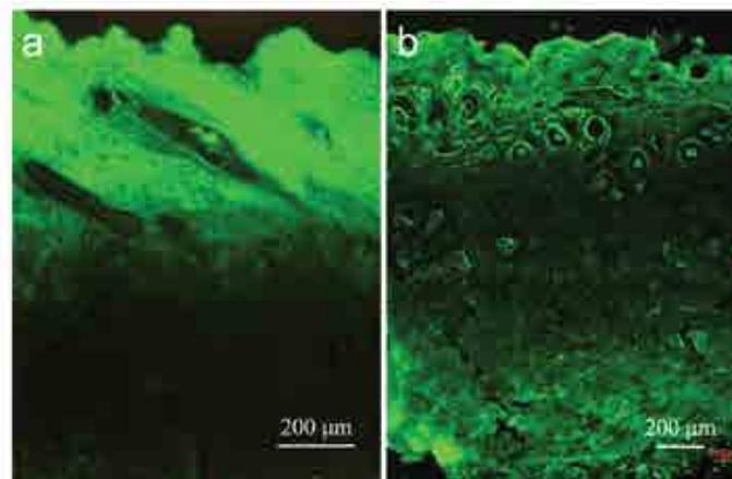
Figure 2. Fluorescence microscopy observation of goatskin treated with FITC-trypsin. (a) one-way diffusion, (b) turbulent diffusion.
