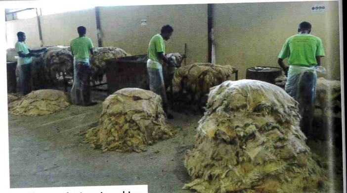
Grading and trimming skins.
