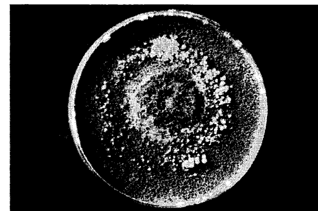
Figure 2. - Trichoderma viride - Specimen covered with growth (rating of 1)
